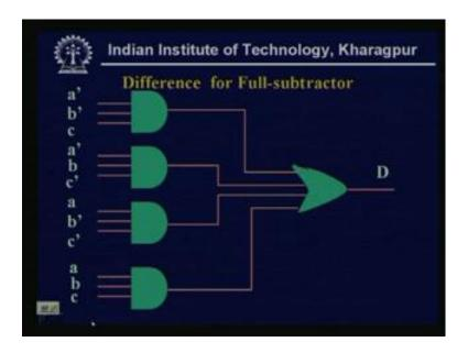
So, if we see that the full subtractor, the difference for full subtractor, then it is totally is same as that of the full adder circuit. Because, that expression same, so already we have discuss this a 4, three input AND gate and 1, four input OR gate is needed.
