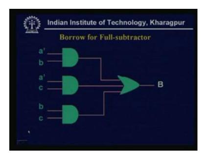
Now, if it is borrow full subtractor, then only the inputs are different, otherwise are structure is totally same. For the first AND gate the inputs are a dash and b one complemented variable is there. For the second AND gate, also one complemented variable a dash is there, for the third word, it is only b c and 1, three input OR gate is
