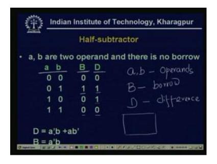
So, just now if I write in the truth table form, that mean a b are the two operands, these are the two operands B is the borrow and D difference. So, a b are the operands B is borrow and D difference, that we want to compute. Now, 0 0 borrow is 0, difference is 0, 0 1, 0 minus 1, this is the situation that, when borrow is 1 difference is 1, 1 minus 0 differences 1, borrow 0, 1 minus 1 difference is 0 borrow 0.
