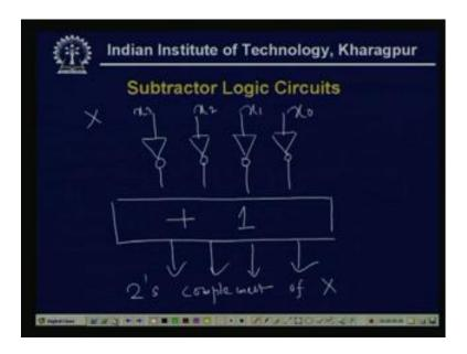
So, the subtractor logic circuit, we can easily draw that because it is a nothing but that addition only the 2's complement we have to do, so if it is 4 bit number, then only some 4 inverter and needed because this is flip or flipping the bits. So, there will be four inputs say this is that  $x ext{ 3, } x ext{ 2, } x ext{ 1 } x ext{ 0 that } X$  is the input and then we add this plus 1 is added and it represents, it represents the 2's complement of X.
