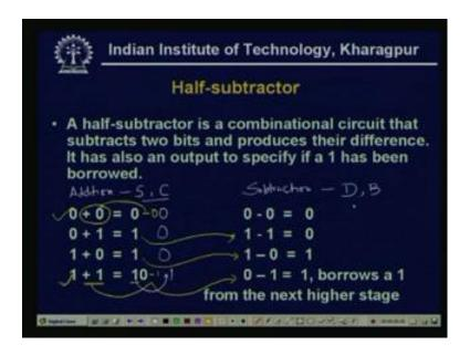
Now, a half subtractor is a combination circuit; that subtracts two bits and produces the difference. It has also an output to specify, if a one has been borrowed, so the similarity with the adders is that, in case of addition, it was for addition, it was the carry signal, for addition one sum and one carry as been generated. For subtraction, that sum replaced by the difference, because it computes the difference and the carry concept is actually they borrow.
