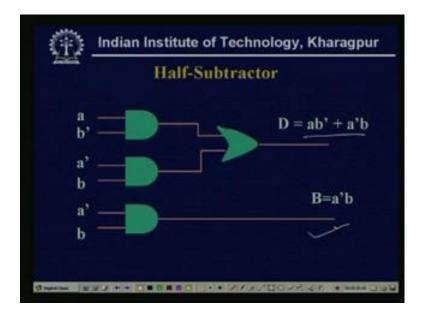
So, half subtractor circuit, again there are there will be two output, one for the difference, one for borrow, already we have seen the difference is same, at the carry of addition operation, that is two input XOR. And, that is AND, OR realization, then a b dash and this is a dash b, the 2, two AND gate and then the output of the AND gate is fade to a two input OR gate. So, this gives you the difference a b dash plus a dash b and the borrow is a dash b.
