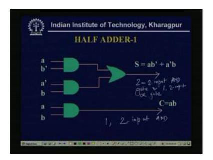
So, if we realize the realization is very simple because a b dash plus a dash b and now again assuming, that my complimented as well as uncomplicated variables are literals are available. Then, this is a 2, two input AND gate and 1, two input OR gate, so my S is that to a b dash and a dash b and there are OR, answer this is my S and carry a simple C is equal to a b.
