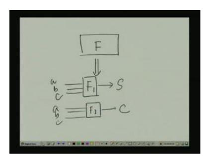
Now, again here they actually the F; that has been partitioned into F 1 sum and F 2 carry a b c are the inputs. So, F 1 means that a b c are the three inputs and the carries the output and a b c are the three inputs and sum is the output, that is F 2.
