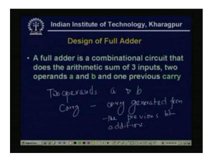
So, this we can tell that the two operands, a and b and the carry is actually the carry generated from the previous bit operation, bit addition. Notice here, that in the half adder we have not considered that thing. So, half adder means mainly the single bit addition and here actually the multi bit addition, so now we see that, how we can design the adder.
