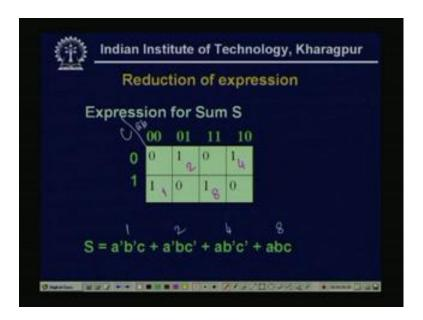
That 1, then 2, 4 and 7, so for 1, 2, 4, 7, see for 1, if I take in this way, so it give this is my a and this is b, then actually this should be a b c, there are three inputs, so this should be a b, this should be c. So, these will be the 1, this is the 2 0, 1 0, then this is 4, this is 8,
