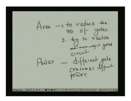
So, mainly the parameters that we have to consider, that one is the area means always we try to reduce the number of gates as well as another point. We can tell that, always we try to realize minimum input gates or gated circuit, means that, if the four input EXOR is needed, then always that. We will use that 3, two inputs EXOR and another is the power.
