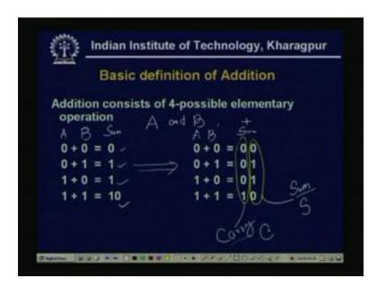
So, as it is name implies the addition consists of the adder, does the addition operator and this consists of four possible elementary operation and these operations, say there are two bits say this is. So, addition we are assuming there are two operands A and B, we are taking the addition, so I am giving the addition notation as plus, now this is my A value and B value.
