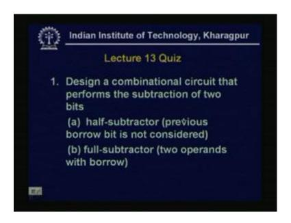
And now the problem is design a combination circuit, that performs the subtraction of two bits, mainly the addition, we have discussed and the subtraction for similar to the half adder and full adder. First we have to do the half subtractor and then it is full subtractor, so first we have to define, what do we mean by half subtractor, half subtractor means that again this will be a single bit minus, where that previous borrow bit, the where the in for addition, it was the carry bit.
