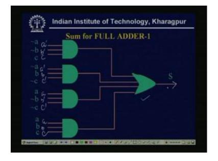
Because, now see the sum was how many 1, 2, 3, 4, 4, 3 input AND gate and 1, 4 input OR gate. Now, see... So, these are the 4 AND gate three inputs AND gate and it is inputs are actually a dash b dash c, a dash b is c dash, a b dash c dash and a b c. That means both complimented and uncomplicated variables are available and 1, 4 input OR gate, so this gives a sum.
