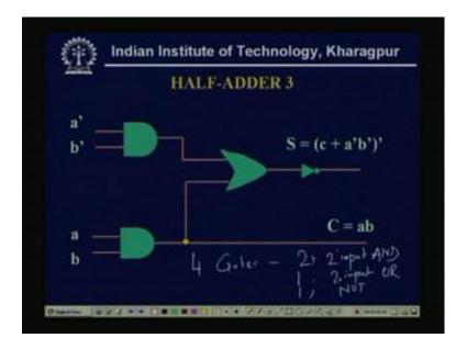
Now, see here only 4 gates are needed, if we do this type of realization, then my half adder circuit takes only 4 gates, that 2, two input AND gates 1, two input OR and 1, NOT. So, totally inputs are only 4, initially it was 17 inputs, always we are assuming in the all the circuits, we are assuming that the variables are available both in complemented and uncomplimented form.
