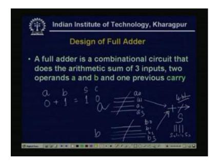
Now, we see design of a full adder, now a full adder is a combination circuit, that does the arithmetic sum of three inputs, two operands a and b and one previous carry. Now, what do we mean by this, see earlier in the half adder, we have only taken two operands a b, this is 0, a is 0, say b is 1 and it is adding 1, sum is 1 and carry is 0, now this is simple two input or you can take single adder.
