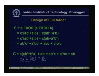
So, just remember the previous one previous1, that see this is c this is actually the c and this is a EXOR b with a b. So, see this is C AND, here 1 AND gate is needed, one, two input EXOR gate is needed and for this a b 1, again this is a two input AND gate.
