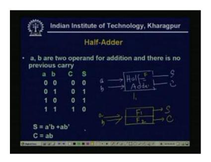
So, given these problem of addition, now how we can write my adder, say if it is, I am considering 1 half adder and the half adder. We define as if there are two operands for addition and there is no previous carry; that means, only two values are added and the operator already operation, we have defined. So, here as if we are now identifying that, there are two operands, a b there are the inputs.
