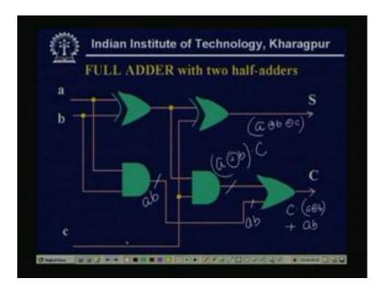
So, what we have done, say this C that this equation is mainly doing that thing, so this is a b, actually this AND input is a b, and this AND in output, this is one input is a EXOR b ended with c. And this is a b, so this c is C dot a EXOR b plus a b, so this is one
