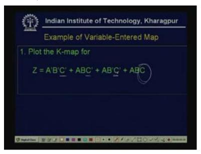
We take one example, so plot the K map for Z equal to A dash B dash C dash, plus A B C dash, plus A B dash C dash plus A B C.
