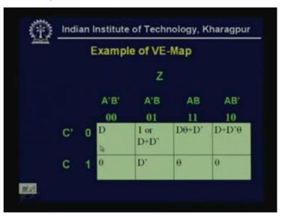
See, A B C 0 0 0 means, A dash B dash C dash, this is my term 0 0 0 and, see if D is 0, output is 0, Z is 0, if D is 1, Z is 1. That means, my output is nothing but the D, so for this, that A dash B dash C dash, this is D.
