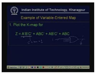
See, the previous example A dash B dash C dash exist, see here A dash B dash C dash is one of the minterm. So, that means, if A dash B dash is true and C dash is also true, means C dash equal to 1. Then the output will be 1, because this is a sum of minterms, that means, again if we realize, this is nothing but a four input OR gate and if anyone of the OR gate is 1, anyone of the input of the OR gate is 1, then it will be, output will be 1, so this Z will be 1.
