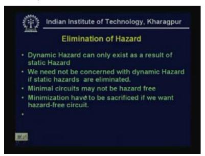
So, dynamic hazards can only exist as a result of static hazards and we need not be concerned with dynamic hazard, if static hazards are eliminated. So, that means, in the previous cases ((Refer Time: 33:01)) that if, if this glitch are not there, then, there will be no glitch in the H also, so in the H also, there will be no glitch. Now, if we summarize that, the hazards covers by K map, then what we get that, the minimum circuits may not be hazard free.
