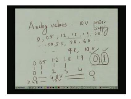
See, I have some analog, again if we take the same example of that power supply that is a one the analog values can be 0 if it is a say 10 volt power, it can take 0 or 0.5 volts then 1.2 volts it can be, then it can be 1.8 volts, 1.9 volts, 2.0 volts like that, like it can be 5.5. So, it can be 5.0, 5.5, 5.8 like 6.0 in that way in that way it will be say 9.8, then 10 volts.
