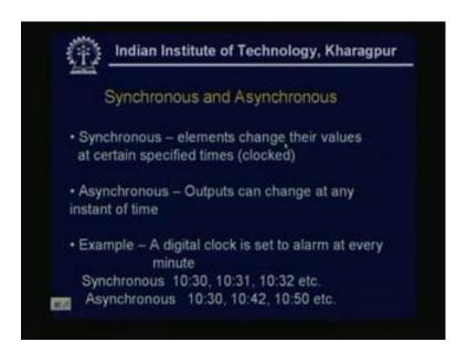
Now, another two terms are very important, when we read that digital systems, one is called synchronous another is called asynchronous. So, what do you mean by synchronous system? A synchronous system has the is the elements, if the elements change their values at certain specified times. Certain specified times means some specific times only they can changed and it is normally we call that clocked, we will discuss that thing later.
