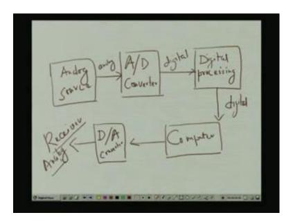
And I again I do that this is my that one analog of source, now I want one converted this is called analog to digital converter we normally called a 2 D converter. And then, so here it is a analog signal here output is digital. So, now, can easily attach one digital system, so some digital amplifier I am telling, I earlier it was analog amplifier, so better I call some digital processing, so this is an digital processing.
