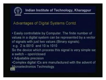
Now, easily controllable by computer this is the main advantage of the digital systems, so the finite number of values in a digital system can be represented by a vector of signals with just two values, what we call the binary signals. Let us discuss this point, because this is the main backbone of the digital systems, so already we have defined that a digital system that it is the system where it can take only some finite values.
