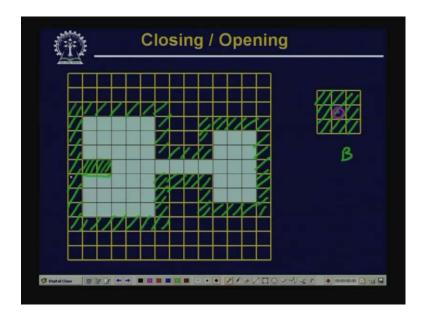
The effect will be something like this that these internal noisy points we have assumed, these will be filled up but simultaneously, the boundary of the object will also be expanded by one pixel all around the boundary. So, this is what the dilation output that I am going to have. So, this is the dilation output, all these pixels will turn out to be object pixels.
