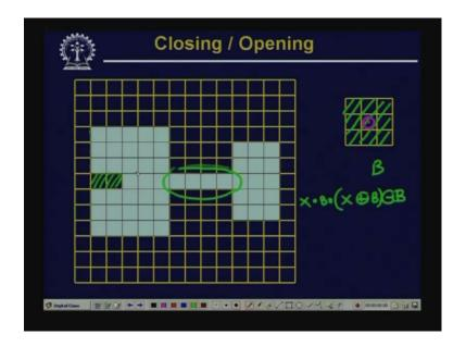
Butthe other noise that is this one where two different object regions have been connected by a thin line which is one pixelwhite that has not been removed. So, in order to remove this,I do the inverse operation.That is first I apply the erosion and by applying the erosion,I will have reduction in the object region.Tocompensatefor this reduction,I will have the subsequent dilation operation.And, this erosion and dilation will also be done by the same with respect to the same structuring element.
