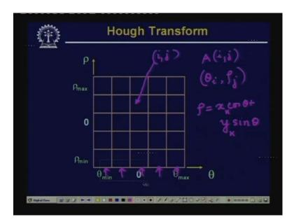
So for computation, again here, what we have to do is we have to define it, the rho theta space into a number of accumulator cells. So, the accumulator cells are given like this as in this figure. So, here again, any ij'th accumulator cell, an accumulator cell say (i, j) this ij'th accumulator cell
