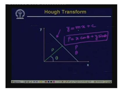
So here again, I have this straight line in the xy frame. But instead of taking the slope intercept form where the equation was given by y is equal to mx plus c, I take the normal representation where the equation of the straight line is given by rho is equal to x cosine theta plus y sin theta.
