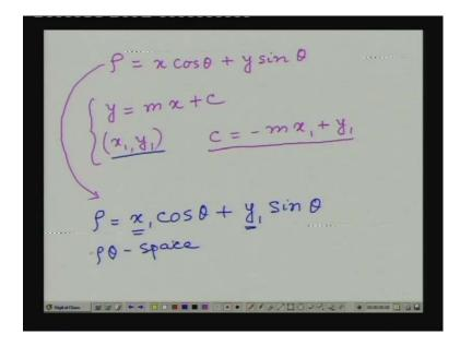
Now, in this particular case, our equation of the straight line is taken as rho equal to x cosine theta plus y sin theta whereas in our earlier case, our equation was y is equal to mx plus c. So, here, you will find that in this particular case, given a single point say  $(x_1, y_1)$  in the spatial domain in the parameter domain in the mc plane, the corresponding equation becomes c is equal to minus m  $x_1$  plus  $y_1$  which is again the equation of a straight line.
