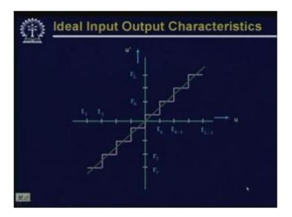
So, let us come to this particular slide. So, it shows the input output relationship of a quantizer. So, it says that whenever your input signal u, so along the horizontal direction we have put the input signal u and along the vertical direction we have put the output signal u prime which is the quantized signal.
