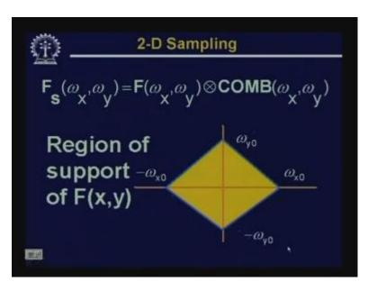
So, coming back to similar concept as we have done in case of 1 dimensional signal X (t) that  $F_s$  omega x omega y which is now the convolution of F omega x omega y which is the frequency spectrum of the original image convoluted with comb omega x omega y where comb omega x omega y is the Fourier transform of the sampling function in 2 dimension.
