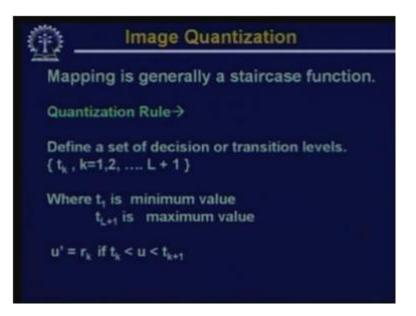
Now, this quantization is a mapping which is generally a staircase function. So, for quantization what is done is you define a set of decision or transition levels which in this case has been shown as transition level  $t_k$  where k varies from 1 to L plus 1.
