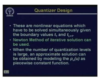
Now, you find that these 2 equations are non linear equations and we have to solve these non linear equations simultaneously, given the boundary values  $t_1$  and  $t_L$  plus 1. And for solving this, one can make use of the Newton method, Newton iterative method to find out the solutions.
