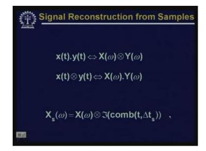
The convolution theorem says that if we have 2 signals X (t) and y (t) in time domain, then the multiplication of X (t) and y (t) in time domain is equivalent to if you take the convolution of the frequency spectrum of X (t) and frequency spectrum of y (t) in the frequency domain. So, that is to say that X (t) into y (t) is equivalent to X omega convoluted with Y omega.
