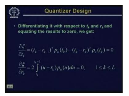
So, if I differentiate this particular error value - u minus  $r_i$  square  $p_u$  (u) du, integration from  $t_i$  to  $t_i$  plus 1; in that case what I get is zeta is the error value del zeta del  $t_k$  is same as  $t_k$  minus  $r_k$  minus 1 square pu  $t_k$  minus  $t_k$  minus  $r_k$  square pu  $t_k$  and these has to be equated to 0.
