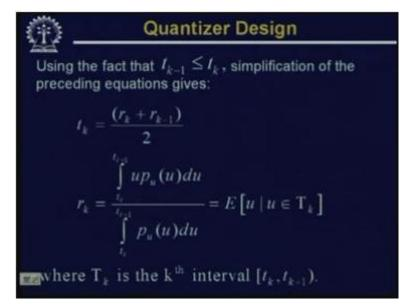
Now, by solving these 2 equations and using the fact that  $t_k$  minus 1 is less than  $t_k$ ; we get 2 values. One is for transition level and the other one is the for the reconstruction level. So, the
