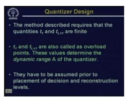
Now, for solving this particular equation, the requirement is that we have to have  $t_1$  and  $t_L$  plus 1 to be finite. That is the minimum transition level and the maximum transition level, they must be finite. At the same time, we have to assume  $t_1$  and  $t_L$  plus 1 a priory before placement of decision and reconstruction levels.
