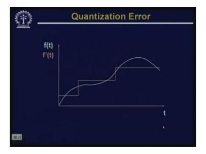
So, to have a clear figure, you find that in this, the green curve, it shows the original input signal and this red staircase lines, staircase functions, it shows that what is the quantization signal quantized signal or **f** at f prime t.
