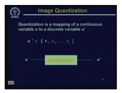
Now, this quantization is a mapping of the continuous variable u to a discrete variable u prime where u prime takes values from a set of discrete variables.
