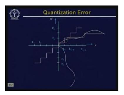
So, here we have plotted the same signal. So, here we have shown the signal is plotted in the vertical direction so that we can find out what are the transition levels or the part of the signal which is within which particular transition level. So, you find that this part of the signal is in the transition levels at  $t_k$  minus 1 and  $t_k$ .
