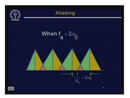
Now, what happens if the sampling frequency is less than twice of omega naught? In that case, as it is shown in this figure; you find that subsequent frequency bands after sampling, they overlap and because of this overlapping, a single frequency band cannot be extracted using any of the low pass filters.
