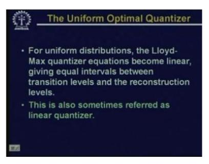
So, for uniform distributions, the Lloyd-Max quantizer equations becomes linear because all the equation that we have derived earlier they are all linear equations giving equal intervals between
