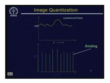
Now, what is this quantization? You find that after sampling of a continuous signal, what we have got is a set of samples. These samples are discrete in time domain. But still, every sample value is an analog value; it is not a discrete value.
