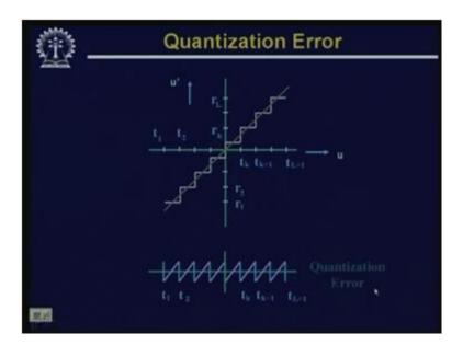
So, here we have shown the same figure. Here you find that whenever this green line which is inclined at 45 degree with the u axis crosses the staircase function; at this point, whatever is your signal value, it is same as the reconstructed value.
