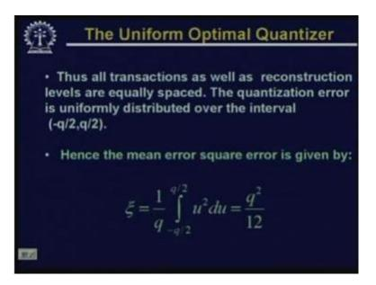
So, here you find that all the transactions, all the transition levels as well as the reconstruction levels are equally spaced and the quantization error in this case is uniformly distributed over the interval minus q by 2 to q by 2. And the mean square error in this particular case if you compute, will be given by 1 upon q u square du you take the integral from minus q by 2 to q by 2 which will be nothing but q square by 12.
