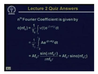
And this term, you have to take the summation from n equal to minus infinity to infinity where the c n f<sub>0</sub> that is the n'th Fourier coefficient is given by the expression c n f<sub>0</sub> equal to 1 upon t<sub>0</sub> then integral v (t) e to the power minus j 2 pi n f<sub>0</sub> t dt where this integration has to be taken over the period t<sub>0</sub>.
