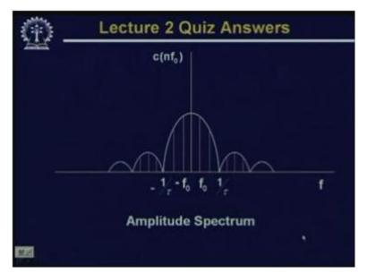
And if I plot this, the plot would be something like this where we have plotted c n  $f_0$  versus A f and this will be a line spectrum where I get lines at f equal to 0, f equal to  $f_0$ , f equal to twice  $f_0$  and so on and the those components will vary the envelop of this frequency components will follow the sin c function.
