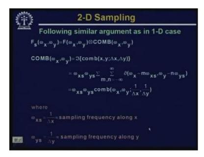
So, as we have done in case of 1 dimensional signal; if we want to find out the frequency spectrum of this sampled image, then the frequency spectrum of the sampled image  $f_S$  omega x omega y will be same as f omega x omega y which is the frequency spectrum of the original image f (x, y) which has to be convoluted with comb omega x omega y where comb omega x omega y is nothing but the Fourier transform of comb x y delta x delta y.
