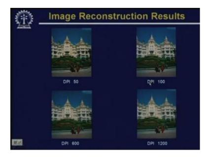
So, let us see some result. This is here we have shown 4 different images. So, here you find that the first image which is shown here was sampled with 50 dots per inch or 50 samples per inch. Second one was sampled with 100 dots per inch, third one with 600 dots per inch and the fourth one with 1200 dots per inch.
