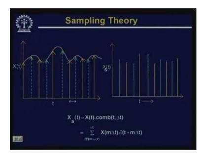
This is a signal X (t) which is a function of a single variable say t. And then, what we have done is we have sampled these 1 dimensional signal with a sampling function which is represented in the form of comb function say comb of t delta t and we get the sample values as represented by  $X_S$  (t) and we have we have also said that this  $X_S$  (t) can be represented in the form of multiplication of X (t) by comb function of t delta t.
