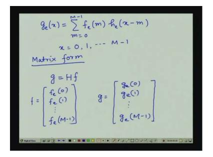
And now, in discrete domain, the convolution function can be written as  $g_e(x)$  is equal to summation  $f_e(m) h_e(x \text{ minus } m)$  where this m will be varying from 0 to capital M minus 1 and x we will assume values from 0 to capital M minus 1. So, this is the discrete formulation of the convolution equation that we have obtained in case of continuous signal cases.
