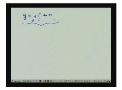
So, in case of 2 dimensional function that is in case of a digital image, we have seen that the degradation model can simply be represented by this expression g equal to H into f plus n where this vector f is a vector of dimension m into n and the degradation matrix H which is of dimension m into n by m into n is actually a block circulant matrix where for each block, the matrix is obtained from the j'th row of the degradation function H (x, y).
