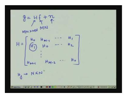
And, if I write this convolution expression in the form of a matrix and incorporating the noise term eta (x, y), I will get a matrix equation which is of the form g equal to Hf plus n where this matrix where this vector f is a vector of dimension capital M into N which is obtained by concatenating different rows of the 2 dimensional function f (x, y) that is the first N number of elements of this vector f will be the elements of the first row of matrix f (x, y).
