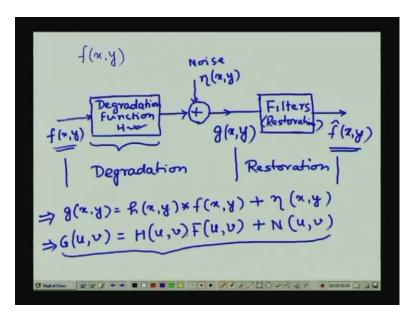
So here, we assume that our input image is image f(x, y). It is a 2 dimensional function as before and we assume that this f(x, y), the input image f(x, y) is degraded by a degradation function H. So, we will put it like this that we have a degradation function H which operates on the input image f(x, y).
