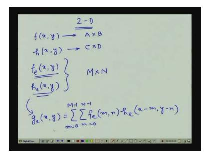
So, let us see what we get in case of 2 dimensional functions that is in case of 2 dimensional images. So, in case of 2 dimension, we have the input function or the image function which is given by f(x, y) and we have the degradation function which is given by h(x, y) and we assume that this if f(x, y) is sampled to an array of dimension capital A by capital B and say h(x, y) is sampled to an array of dimension say capital D.
