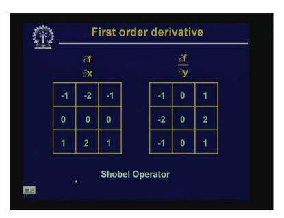
So, for computing the first order derivative along x direction, the left hand side shows the mask and for computing the first order derivative along y direction, the right hand side shows the mask. And later on, we will see that these operators are known as Shobel operator and using these first order derivatives; when we apply these first order derivatives on the images, the kind of processed image that we get is like this.
