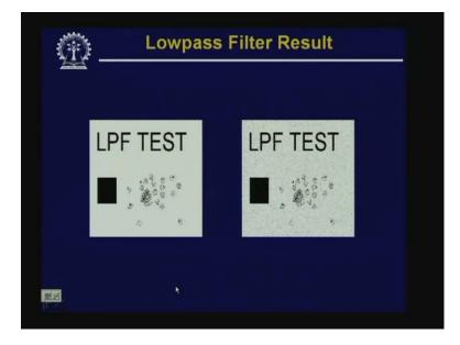
So here, we use 2 images for test purpose. On the left hand side, we have shown an image without any noise and on the right hand side, we have shown an image where we have added some amount of noise.
