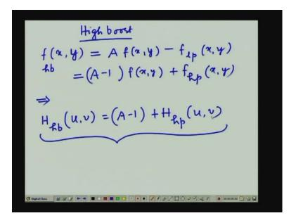
So, there we have said that in spatial domain; the high boost filtering operation, the high boost filtering output f (x, y) if I represent it if I represent this as  $f_{hb}(x, y)$  is nothing but A into f (x, y) minus f  $_{lp}(x, y)$  and which is can be represented as A minus 1 into f (x, y) plus f high pass filtered output (x, y).
