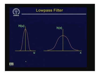
So here, on the left hand side, we have shown the frequency domain filter H (u) as a function of u and on the right hand side, we have shown the corresponding spatial domain filter h (x) which is a function of x. Now from these filters, it is quite obvious that all the values once I specify a filter H (u) as a function of u in the frequency domain, the corresponding filter h (x) in the spatial domain, they will have all positive values.
