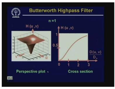
This shows the butter worth filter perspective plot as well as cross section of butter worth filter of order 1 and if I apply such high pass filters to the image to the same image, then the result that will obtained is something like this.
