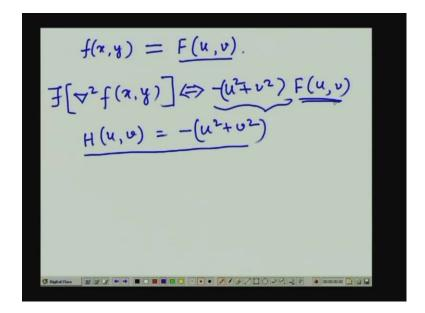
It is simply because if I take the Laplacian of a function; if for a function f(x, y), I get the corresponding frequency domain say F (u, v) the corresponding Fourier transform, then the Laplacian operator if I perform del square f(x, y) and take the Fourier transform of this, this will be nothing but it can be shown it will be equal to minus u square plus v square into F (u, v).
