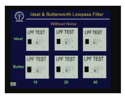
Then, if I process that image using the ideal low pass filter and using the butter worth filter; the top rows shows the results with ideal low pass filter when the image is without noise and the bottom row shows the result by applying the butter worth filter again when there is no noise contamination with the image.
