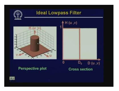
A plot of this kind of function is like this. So, here you find that the left hand side shows the perspective plot of such an ideal filter whereas on the right hand side, we just show the cross section of such an ideal filter and in such cases, we define a cut off frequency of the filter to be the point of transition between H (u, v) equal to 1 and H (u, v) equal to 0.
