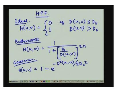
So, just in the reverse way we can define an ideal high pass filter as, for an high pass filter, the ideal high pass filter will be simply H (u, v) is equal to 0 if D (u, v) is less than or equal to  $D_0$  and this will be equal to 1 if D (u, v) is greater than  $D_0$ . So, this is the ideal high pass filter.
