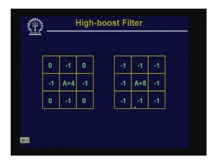
So, using this we can get a similar type of mask where the mask is given by this particular expression. So, using these masks, we can go for high boost filtering operation and if I use this high boost filtering, I get the high boost output as we have already seen earlier.
