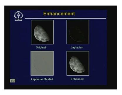
So, the next one shows that if we have this original image, these are that same detailed images that we have shown earlier. On the right bottom, you have the enhanced image or the detailed images are added to the original image and for performing this operation, we can have a composite mask where the composite mask is given like this.
