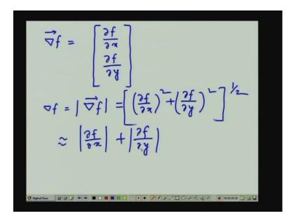
What you used for obtaining the first order derivatives is by using the gradient operator where the gradient operator is given like this. Gradient of a function f as the gradient is a vector, so we will write as a vector is nothing but dell f dell x and dell f dell y. So, this is what gives the gradient of a function f and what we are concerned about for enhancement is the magnitude of the gradient.
