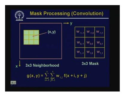
So what we have done is we have the original image f(x, y), we defined a mask corresponding to the type of operation that we want to perform on the original image f(x, y) and using this mask the kind of operation that is done the mathematical expression of this is given on the bottom and if you analyze this, you will find that this is nothing but a convolution operation.
