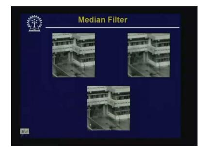
So, there we have said that instead of using simple box filter or the simple averaging filter if I go for order statistics, go for filtering based on order statistics like median filter or the pixel value at a particular location in the processed image will be the median of the pixels in the neighborhood of the corresponding location in the original image; in that case, this kind of filtering also reduces the noise. But at the same time, it tries to maintain the contrast of the image.
