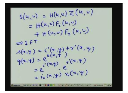
Now, if I define a filter say H (u, v) and apply this filter on this Z (u, v), then the output that I get is say S (u, v) which is equal to H (u, v) times Z (u, v) which will be nothing but H (u, v) times  $f_i$  (u, v) plus H (u, v) times  $F_r$  (u, v).
