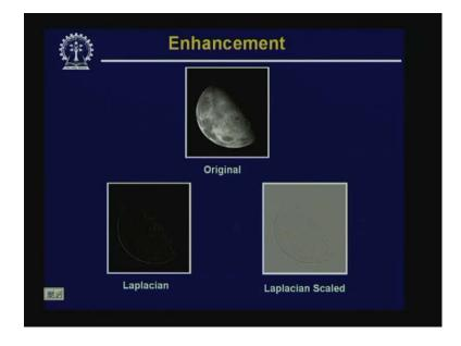
Now, using this Laplacian mask, we can find out the high frequency detailed contents of an image as has been shown in this particular one. Here you find that the original image, when it is processed using the Laplacian mask, the details of the image are obtained on the left hand side. Bottom left, we have shown the details of the image. On the bottom right what we have done is it is the same image which is displayed after scaling so that the details are displayed properly on the screen.
