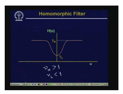
So now, if we define a filter like this a filter response like this and here if I say that I will have say gamma H greater than 1 and gamma L less than 1, this will amplify all the high frequency components that is the contribution of the reflectance and it will attenuate the low frequency components that is contribution due to the illumination. Now, using this type of filtering, the kind of result that we get is something like this.
