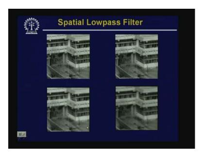
Here also you find that using the low pass filter, the content, the noise in the image gets removed but at the cost of the sharpness of the image. That is when we take the average over a larger mask, a larger size mask; then it helps to reduce the noise but at the same time, a larger mask introduces large amount of blurring in the original image.
