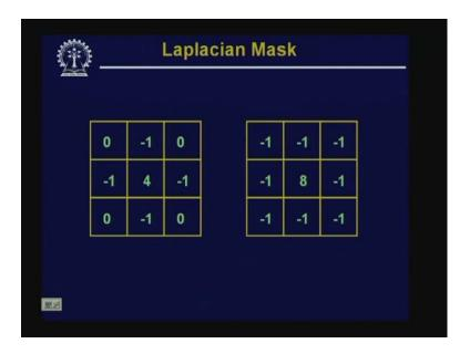
We can also use another type of masks where the center coefficients are positive. You find in case of earlier masks, the center coefficients are negative whereas, all the neighboring coefficients are positive in the Laplacian mask. In this case, the center coefficient is positive whereas, all other neighboring coefficients are negative.
