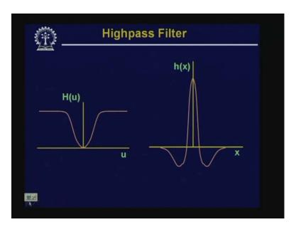
Now, in the same manner, as we have said the low pass filter; we can also make the high pass filters again in the Gaussian domain.
