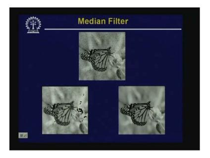
Then this shows another median filter output result. The bottom 2 images on the left side, it is the image obtained using the box filter on the right hand side, it is the image obtained using the median filter. The enhancement using the median filter over the box filter is quite obvious from this particular image.
