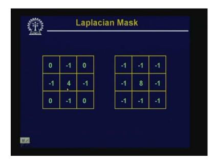
So, the Laplacian mask that we have used, we have seen that the center pixel is having a positive value whereas all the neighboring pixels have the negative values and this is true for both the Laplacian masks if I consider only the vertical and horizontal components or whether along with vertical and horizontal components, I also consider the diagonal components.
