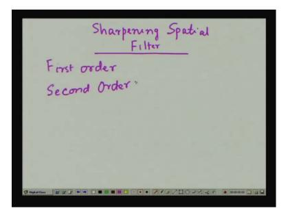
So, we will consider sharpening spatial filter. So, the objective of this sharpening spatial filter is to highlight the details, the intensity details or variation details in an image. Now, through our earlier discussion, we have seen that if I do averaging over an image or smoothing over an image, then the image becomes blurred or the details in the image are removed. Now, this averaging operation is equivalent to integration operation.
