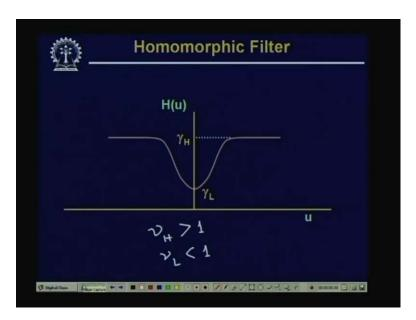
So, we have to have some scaling operation because I will have say gamma H greater than 1 and gamma L less than 1. This will amplify all the high frequency components that is the contribution of the reflectance and it will attenuate the low frequency components that is contribution due to the illumination. Now, using this time of type of filtering, the kind of result that we get is something like this.
