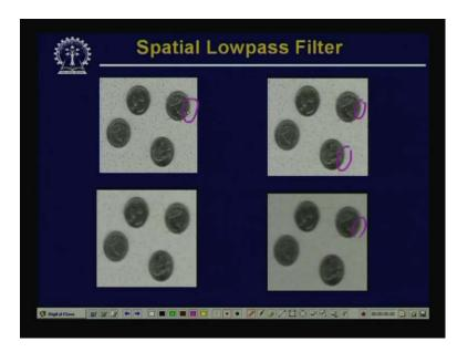
Now, using this kind of mask operation, here we have shown some results. You find that the top left image is noise image. When you do the masking operation or averaging operation on this noisy image, the right top image shows the averaging with a mask of size 3 by 3, the left bottom image is obtained using a mask of size 5 by 5 and the right bottom image is obtained using a mask of size 7 by 7.
