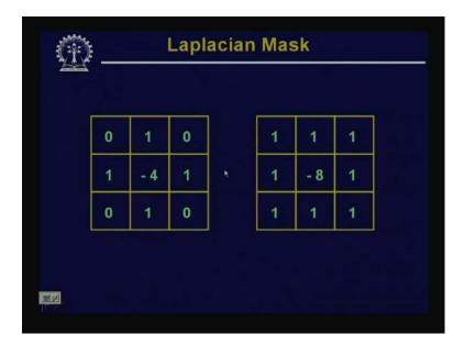
So, on the left hand side, the mask that is shown, this mask considers the Laplacian operation only in the vertical direction and in the horizontal direction and if we also include the diagonal directions, then the Laplacian mask is given on the right hand side. So, we find that using this particular mask which is shown on the left hand side, I can always derive the expression that we have just shown.
