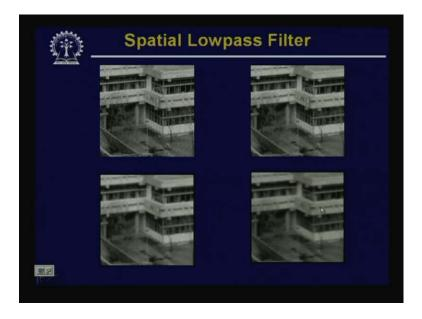
So, here is another image. Again, we do the masking operation or the smoothing operation with different mask sizes. On the top left, we have an original noisy image and the other images are the smoothed images using various mask sizes. So, on the right top, this is obtained using a mask of size 3 by 3, the left bottom is an image obtained using a mask of size 5 by 5 and the right bottom is an image obtained using a mask of size 7 by 7.
