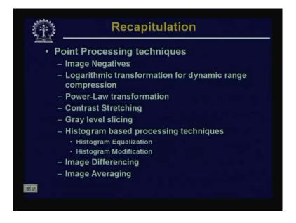
So, what we have done till now is the point processing techniques for image enhancement and under this, the first operation that we have done is image negatives and there we have seen that image negative operation is useful incase the image contains information which are either contained in the gray level or in the white pixels that are embedded in dark image regions.
