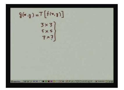
Now, in our earlier discussions we have mentioned that while going for this contrast enhancement, what we basically do is given an input image say f(x, y), we transform this input image by a transformation operator say T which gives us an output image g(x, y) and what will be the nature of this output image g(x, y) that depends upon what is this transformation operator T.
