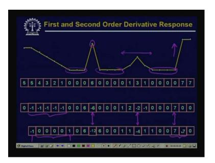
So, this is a 1 dimensional signal where the values of the 1 dimensional signals for various values of x are given in the form of an array like this and the plot of these functional values, these discrete values are given on the top. Now, if you take the first order derivative of this as we have just defined, the first order derivative is given in the second array and the second order derivative is given in the third array.
