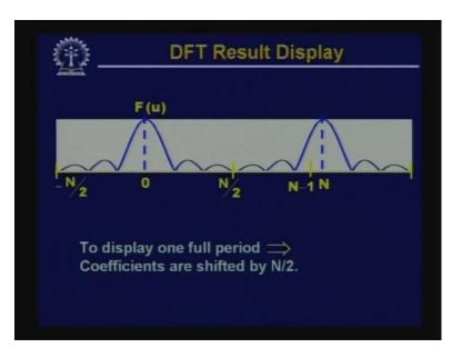
You will find that this is the typical this is a typical Fourier transform of a particular signal and here you find that this Fourier spectrum, the Fourier's transform is centered at the origin and if you look at the frequency access; so this is the u access, if you look at this frequency access, you will find that F of minus u, the magnitude of F of minus u is same as the magnitude of the F of plus u.
