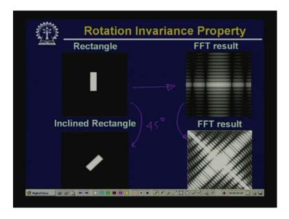
So here, you find that we had a rectangle, an image where we have all values we have pixel values equal to 1 within a rectangle and outside this, the pixel values are equal to 0 and the corresponding Fourier transformation is this. So here, the Fourier transformation coefficients or the Fourier spectrum is represented in the form of intensity values in an image. The second pair shows that the same rectangle is now rotated by an angle 45 degree.
