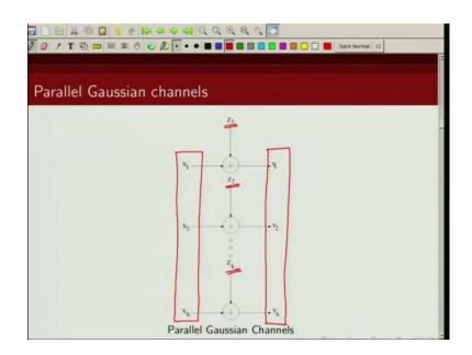
So, as I said this is how a my parallel Gaussian channel looks like I have these inputs X 1, X 2 and X K and these are my output Y 1, Y 2, Y K the noise samples are independent denoted by Z 1, Z 2, Z K.
