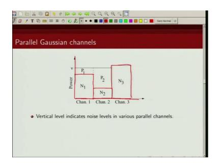
Now, this can be visualized in this fashion. So, let say on the x-axis, I am plotting these key channels. So, I have this channel 1, channel 2, channel 3 like that I am plotting. And here I am plotting power. So, initially I plot the noise power. So, if you see this level high, it means the noise level is higher. So, noise level of N 1 is more than N 2, but it is less than the noise in the channel 3, so that is what this height of this N 1 into N 3 means.
