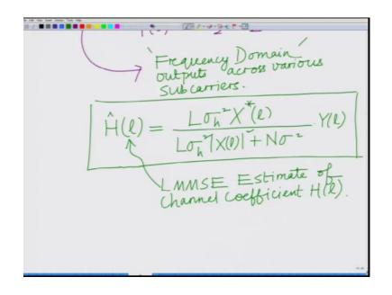
Well we have H hat that is what we have derived in 1 of the previous modules H hat 1 equals L sigma H square X conjugate 1 divided by L sigma x H square magnitude X 1 square plus N sigma square into y 1, this is the LMSSE estimate of channel coefficient H 1.
