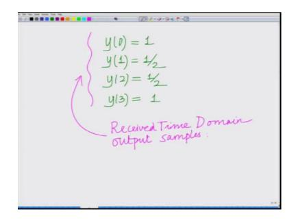
So, let us continue with this example let us consider the received symbols, received time domain samples, received time domain samples to be given as - the domain output sample as y 0 equals 1 y 1 equals half y 2 equals half y 3 equals these are the received time domain, these are the received time domain output samples. Therefore, the corresponding frequency domains symbols (Refer Time: 01:31) across the various sub carriers are given by the FFT of this time domain samples that is what we feel.
