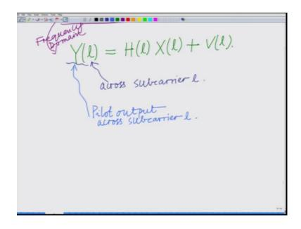
What are these y l's these y l's are the symbol pilot output received across the pilot outputs that are received across the sub carrier, across the sub carrier l. So, we have capital y l which is the pilot output received across sub carrier l.
