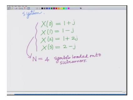
These are the 4 symbols these are the N equal to 4 symbols loaded on to the sub carriers these are the n equal to 4 symbols which are loaded on to the 4 sub carriers correct.
