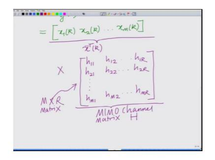
Where x bar k is a transmit vector at time instant k, times the product  $h \ 1 \ 1 \ h \ 1 \ 2$  so on to  $h \ 1 \ r \ h \ 2 \ 1 \ h \ 2 \ 2$  so on up to  $h \ 2 \ r \ h \ m \ 1 \ h \ m \ 2$  so on up to  $h \ m \ r$ . This is your mimo channel matrix h and you can clearly see this is an m cross r. So, we have now the m cross r mimo channel matrix h correct, where m is the number of transmit antennas r is the number of receive antennas correct
