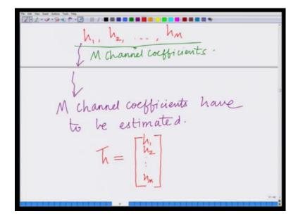
These are the, these are your m channel coefficients, correct. In this wireless, in this multi antenna wireless communication system, we have m channel coefficients, and to begin with, these m channel coefficients are unknown; that is the paradigm of channel estimation. Therefore, this m channel coefficients can now be stacked as a vector. This can be considered as a vector h bar, and that channel vector h bar has to now be estimated. Therefore, this leads to vector parameter estimation.
