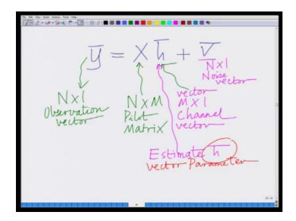
And, of course, this we have already seen before. This is h 1, h 2, h m. This is, which is the pilot, which is the channel coefficient, the channel vector h bar. This is the noise vector v bar, which contains the N noise coefficients v 1, v 2, v N, corresponding to the N received samples y 1, y 2, y N. And now, therefore, if I write this entire thing together
