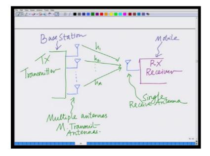
And, in this example, again, similar to our example previously, let us look at the channel estimation. Let us look at, remember the estimation of the fading channel coefficient in the wireless system is known as channel estimation. However, let us look at channel estimation in a multi-antenna system.
