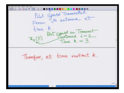
So, let us consider the transmission of pilot symbols. However, I have been slightly inaccurate, because we have multiple antennas. So, we need the transmission of one pilot symbol from each transmit antenna. So, rather than the pilot symbols, we will actually be transmitting pilot vectors, where the vector of transmitted symbols corresponds to one transmit symbol from each transmit antenna.
