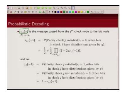
So we are denoting by  $R_{ji}$  the message which is passed from j parity check note to the i<sup>th</sup> bit, we are denoting this by  $R_{ji}$  so what is r,  $R_{ji}$  is the probability that j<sup>th</sup> check note is satisfied given x is + 1, so this is a probability that j<sup>th</sup> check note is satisfied given  $C_i$  is 0 and other bits are given by distribution given by this q, now what is this q distribution?
