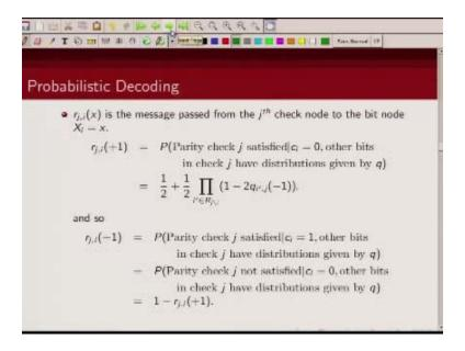
So as we have said before we are writing, we are representing this LDPC code using this stenograph and there are 2 types of information which are getting propagated. One is one sort of messages which is from the message notes going to the variable, going to the parity check notes and this one set of message which from the parity check notes coming back to the message notes.
