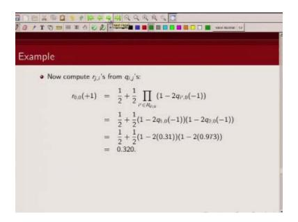
So once we have computed this  $q_{ij}$  the next thing that we need to do is these parity check constraints are now going to check okay given that the bit is zero. What is the probability that parity checks constraint is satisfied, given the bit is one what is the probability that parity check constrain is satisfied?
