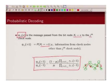
$q_i$ 's are message passed from  $i^{th}$  bit to the  $j^{th}$  parity check constraint. So if you label your nodes from 0,1,2,3,4 as similarly label parity check constraints, so what you are going to notice is so you need to compute your  $q_i$ 's for, for in this example.
