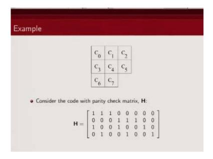
So let us take an example to illustrate the decoding algorithm, so we have a low density parity check matrix given by this we have eight coded bits.
