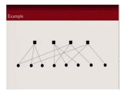
This is the tanner graph corresponding to the parity check matrix, we can just quickly check it.
