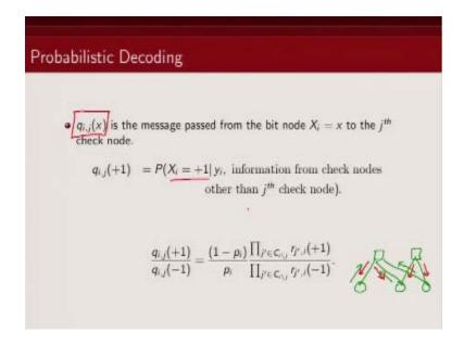
And this is so  $q_{i,j}$  here being +1 is given by what is the probability that  $x_i$  is +1 given receive sequence  $y_i$  and information from parity check nodes other than the  $j^{th}$  parity check node so, what is happening is when you are decoding because each bits are participating in multiple parity check equations, so you are getting some independent information from other parity check nodes and that information you want to pass it to and spread it around in this network.
