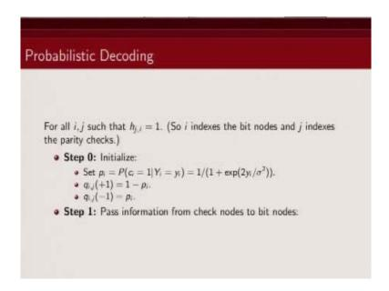
Next is once these messages are sent to check nodes then check nodes will do local computation and it will send this  $r_{i's}$  back to the bit node.
