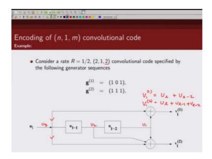
That we are considering we have one input we have two outputs output depends on pass two inputs so basically memory order is two  $g^{(1)}$  is give by this  $g^{(2)}$  is give by this these are my output  $v_1^{(1)}$ ,  $v_1^{(2)}$  these are my output sequences.
