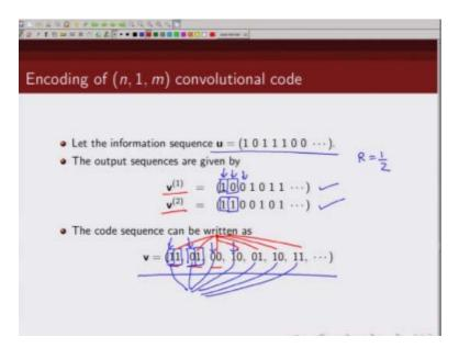
this one this is the output from the first code sequence and what is the output form the second sequence which is this one so what are you doing when your combining these output sequence which is  $v^{(1)}$  and  $v^{(2)}$  so your taking  $v^{(1)}$  like as it is only things is, is this spread out after every second bit and
