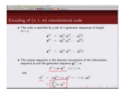
Is a discrete convolution of the information sequence with this generator sequence? So if my generator sequence if my code as memory m then basically I can write this discrete convolution in this particular position and that is basically my output sequence which is discrete convolution of the input sequence with this generator sequence. Now let us take an example
