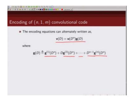
Particular form where output sequence is give by  $u(D^n)$  times g(D) where g(D) is this a generator sequence for the first coded sequence the generator sequence form the second delayed by one generator sequence of the third delayed by two generator sequence of the n delayed by  $D^n$  so the overall encoding sequence can be equivalently written like this.
