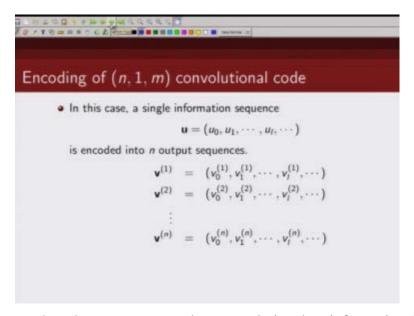
Now we are going to show how we can encode a convolutional an informational sequence using a rate 1/n convolutional encoder.
