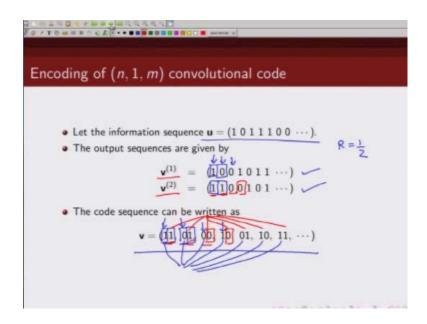
$v^{(2)}$  is delayed by one and it is also spread out this is one this one is appearing here this zero is appearing here this is appearing here so every second bit is also from this encoded sequence and note that this is delayed by one corresponding to  $v^{(1)}$  so that is what we are doing.
