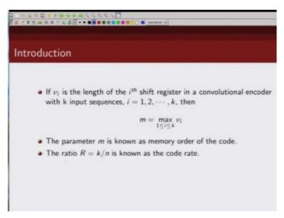
As we know this ratio of information bits to coded bits k/n is known as code rate which we denote by R.
