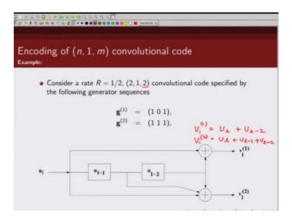
First coded sequence is u<sub>1</sub>+ u<sub>1-2</sub> and the second coded sequence is u<sub>1</sub>+u<sub>1-1</sub>+u<sub>1-2</sub>.
