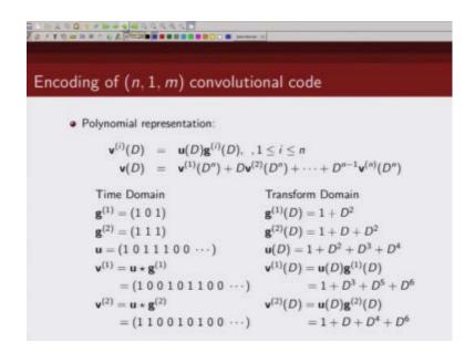
Now we are going to give a polynomial representation of these generator sequence which I very convenient in case of convolutional codes so I'm introducing
