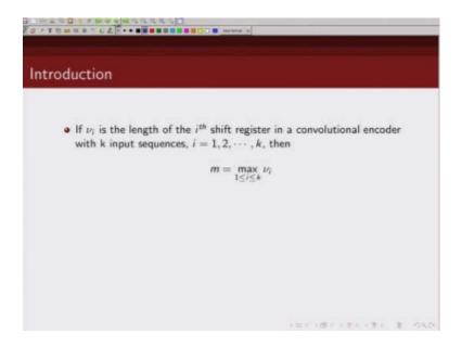
So if we denote by  $\vec{v}$  is the length of the  $i^{th}$  shift register in a convolutional encoder then we defined a memory order as the maximum of maximum length of the shift register among the k shift registers use to represent the convolutional encoder.
