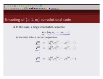
u to be  $u_0$ '  $u_1$ ,  $u_2$ ,  $u_{l-1}$  since is a rate 1/n convolutional code so what we would get is corresponding to one input we are going to get n outputs and we denote these n outputs by  $v^{(1)}$ ,  $v^{(2)}$ ,  $v^{(3)}$ ,  $v^{(n)}$  where each of this  $v^{(i)}$ 's can be return like this
