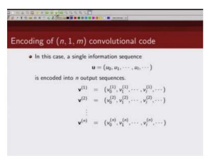
So k is 1 n number of coded bits are send so there is one input coming in and there are n output and the maximum length of this one shift register used to represent this rate 1/n code is m so this shift register as m memory elements.
