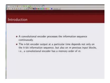
We also know that the output of a convolutional encoder depends not only on the current input put it also depends on past inputs and past outputs depending up on the memory of the convolutional encoder.
