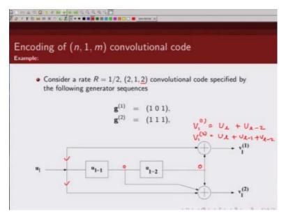
Whatever u0 you had now that u0 has moved here correct and a new bit which is u1 have come here u1 so what is a output at this time it is u1 times g0 +u0 times g1 so I can write.
