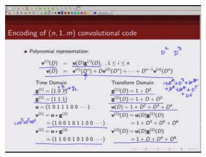
This so if  $v^{(i)}D$  is going to give me output sequence corresponding top each of this output n output outputs now if I can combine this n outputs in this particular section so I take the first output note that I have made a D over in because the if the rate 1/n code the first output will appear after every n bits. The first bit is from the first coded sequence then after n bits it will again repeat it will come meaning so that is.
