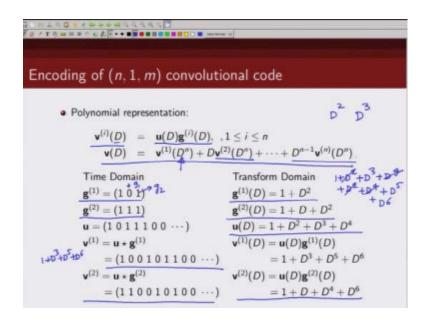
Why I have made it D(n) now how do I combine these n sequences so note I'm take this is output  $v^{(1)} D(n)$  is output from the first code sequence this is the output from the second sequence that is I delayed by one the output from third sequence is delayed by  $D^2$  as similarly the output from the enough sequence it will delayed by n-1 go back here.
