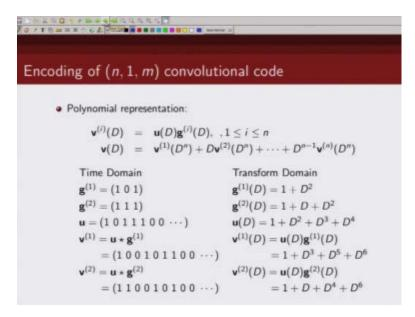
A delay operator D so if you have one memory element delay that will be
