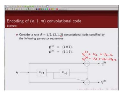
This one which was here when you apply a clock this one moves here and a new bit comes here so now in the next time instance ul-1 becomes 1 and what is ul-2 since ul-1 initially was zero so this zero will come here so the new contents of the shift register will be now one and zero.
