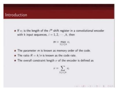
And overall constrains length is defined as  $\Sigma$  of length of all the k shift register that is the overall constrained length.
