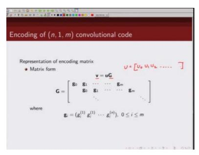
I define this generator matrix G which generate this codes code word so the output code word can be written as input times this generator matrix G okay and this generator matrix is of the from like this so let us just expand it and may be try to explain why the generator form as this semi infinite kind of form for a convolutional code so let us say u is  $u^{(0)}$ ,  $u^{(1)}$ ,  $u^{(2)}$ .... Is continuing set of sequence like this right now what is your, output sequence.
