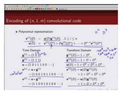
Combined we made it each of this coded bit we made it D forward in next.
