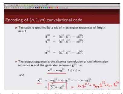
Expand it for this particular example this will be ulg0i+ul-1g1i+ul-2g2i and for the first coded sequence this g is  $g^{(o)}$ ,  $g^{(1)}$ ,  $g^{(2)}$  was 101 and the second sequence was 111 that is why the first.
