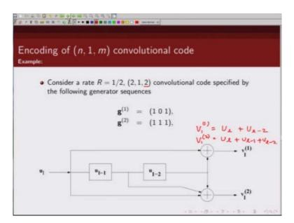
Again go back to this diagram you are input zero here so now this zero will move here and you had a one here so this is one will move here so the new contents which shifty register will be zero and one okay.
