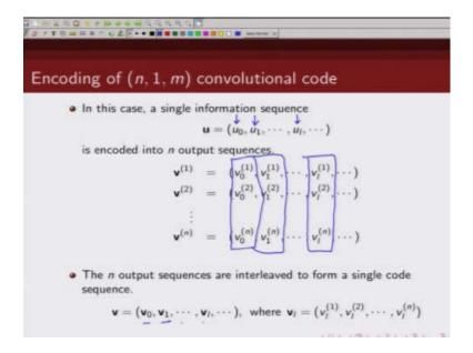
$U_0$  then what is the output these are the n bits output corresponding to this input  $u_0$  similarly corresponding to u1 mu output is this corresponding to u<sub>1</sub> my output is this n bit output okay so I write the output by  $v^{(0)}$ ,  $v^{(1)}$ ,  $v^{(2)}$ ,  $v^{(1)}$  where this  $v^{(1)}$  is a n bit.
