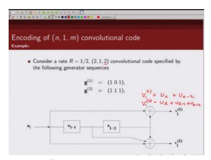
Memory two so you can see  $v^{(1)}l$  this is basically again discrete convolution of input with these generator sequence which we can write as  $ul+u_{1-2}$  and this  $v^{(1)}2$  can be written as ul+ul-1+ul-2 if you go back
