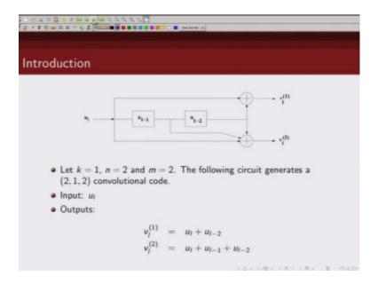
And the output is  $v^{(l)}1$  and  $v^{(l)}2$  and how is  $v^{(l)}1$  and  $v^{(l)}2$  depend on u(l) and the pass values this is given by the interconnection.
