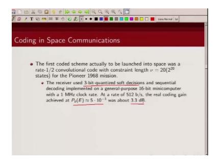
3 bit quantized soft decision and it was implemented on 16 bit minicomputer it provided a coding again of roughly 3.3 so it got a like for a probability for around this it give a coding again for about 3.3 dB
