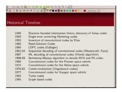
So we know 1948 Shannon founded information theory, and then sub sequently around 1955 Elias came with convolutional codes around 1960's Reed Solomon code and LDPC codes for discovered and around 61, 63 was Wozencraft and Fano came of a sequential decoding of convolutional code which allowed us to decode convolutional code very large memory order 1960 someone 68 Viterbi algorithms for maximum likely would decoding of convolutional code came and then on 74 BCG are algorithm was proposed.
