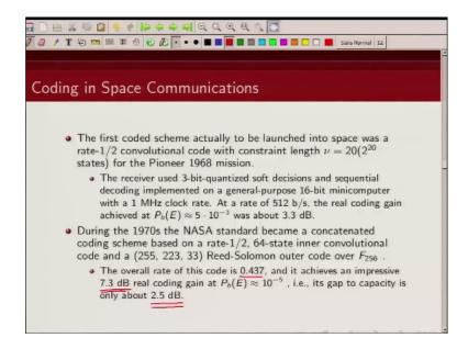
Half convolutional code and it found lot of applications the overall code rate of this was .43 and it a gab to capacity was only 2.5dB it provided coding again around 7.3 dB at bit a rate of 10<sup>-5</sup>
