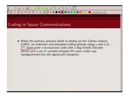
$2^{14}$  state convolutional code assigner code and Reed Solomon code as outer code and a big viterbi decoding viterbi decoding algorithm was prospected which could work over such a large number of sates
