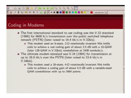
For a 33 kb/s transmission they use a 16 state four dimensional trellis codes modulation scheme and.
