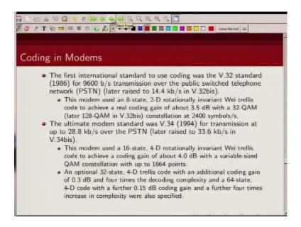
And there was an optional 32 state 4 dimensional trellis code which as all specified in this standard but when we progress to digital backbones then,, then basically there was no need for these codes and so the v 90 v92 standers says essentially do not use any of these coding techniques but in mid 80's and eerily 90's there was lot of they are very successfully these codes where applied for coding for modems.
