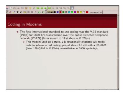
So some of the applications have listed here so initially we had 9.6 kb/s transmission that uses a an eight state code then finally.
