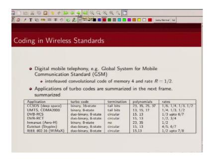
So I like to conclude basically with a giving some examples of communications systems so our GSM use a convolutional code of
