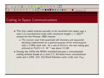
Next around 70's NASA started using this concatenated code outer code was a Reed Solomon code and inner code was 64 state convolutional code rate
