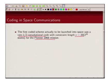
Now pioneer mission was 1968 and they use a rate of convolutional code which as constrained length of 20 so there were 2 to out 20 states and they use sequential decoding
