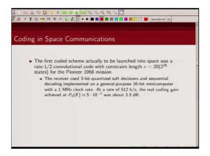
To decode this code the receiver used a
