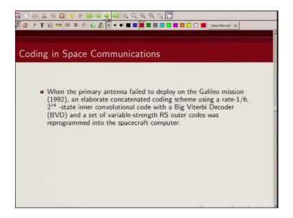
Another big development was when in Galileo's mission this antenna failed to deploy a primary antenna when it fail to deploy so there was an elaborate concatenated coded scheme which used a.
