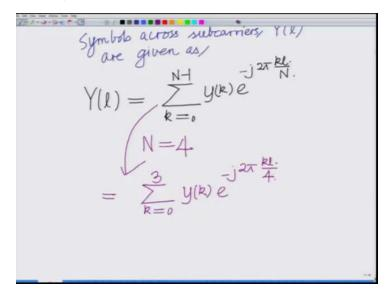
The symbols across the subcarriers Y L are given as; well we can write the expression for that Y L equals well this is similar FFT of the, this k equals 0 to N - 1, y k e power - j 2 pie k L by N and this is the expression for general FFT of length L. So now we have to set N equal to 4 which is the number of subcarriers of frequency points in our system which is equal to.
