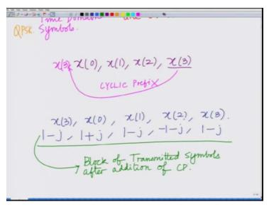
So this is the your basically and we have seen this also many times before, so this is the cyclic prefix. So in the sense that we are adding the cyclic prefix prior to transmission, it is similar to OFDM.
