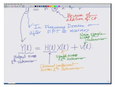
This is basically given as Y of L equals circular convolution becomes multiplication X L + V L and therefore this Y L is the output coefficient output across your Lth from carrier, H L is the channel coefficient across Lth subcarrier, this is the channel coefficient across Lth subcarrier.
