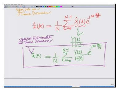
The x hat x is the IFFT of the capital X hat of L e to the power of j 2 pie k L by N. And now we know this X hat of L is basically equal to Y of L divided by H of L. So which I can substitute now, so this is basically 1 over N your submission L equal to 0 to N - 1 Y of L divided by H of L times he to the power e to the power of j 2 pie k L by N.
