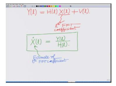
Yeah, Y L equals H L times X L +V L. And therefore, X hat L X hat of L, this is the estimate of the Lth FFT coefficient. This is the estimate of the Lth FFT coefficient, this is equal to Y L which is the output which is output sample across the Lth subcarrier and capital H L which is the channel coefficient across the Lth subcarrier therefore, if you do Y L divided by capital H L, you get the estimate capital X hat L.
