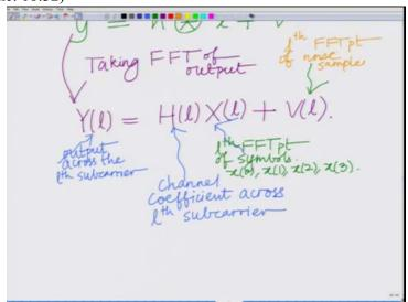
This is across the subcarriers yeah, taking the FFT across the Lth subcarrier in fact, Y L is the output symbol across the Lth subcarrier, H L is the channel coefficient across the Lth subcarrier, X L is basically your symbol transmitted on the that is basically, now this is basically not the symbol on the Lth subcarrier, but this X L is the Lth FFT point of the symbols.
