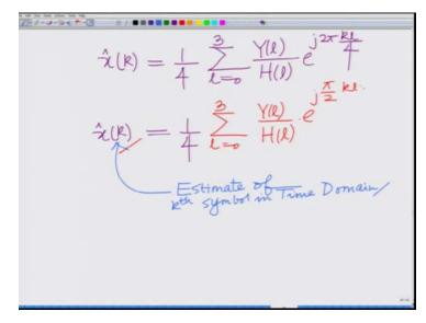
L equal to 0 to 3 Y L divided by H L e to the power of j 2 pie k L divided by 4, which is basically, you can write this as your x hat of k equals 1 over 4 submission L equal to 0 to 3 Y L divided by H L e to the power j 2 pie e to the power of j in fact, I can directly write this as pie over 2 k L, okay.
