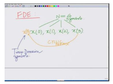
These are not the samples, but these are in OFDM, these are the small x in OFDM are the time domain samples which are generated by the IFFT of the symbols loaded onto the subcarriers. However, in FD we directly trough with the symbols, there is no there is no loading of the symbols on the subcarriers instead of that, the small x, small x 0, small x 1, small x 2, small x 3, these are the symbols.
