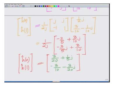
That is, 1 over 2 j times (())(28:02) the diagonal elements negative of the of diagonal elements. So this is the inverse of the matrix, this times half j 3 by 10 - 1 by 10 J.
