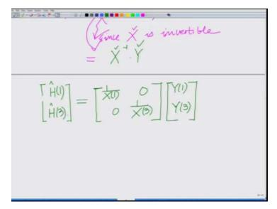
Since X check is invertible this is basically equal to your X check inverse times Y check and since X check inverse is diagonal, the inverse of X check is simply the inverse of the diagonal elements that is 1 over X 1, 1 over X 3 times Y 1 Y 3 and this is basically your estimate. This is your estimate of the channel coefficients. Therefore, now I can calculate the estimate H hat 1 as simply that is your Y 1 divided by X 1.
