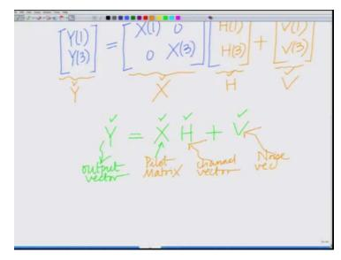
Y 1 Y 3 equals X 1 X 3, the diagonal matrix times this vector H 1 H 3 of channel coefficient + V 1 V 3.
