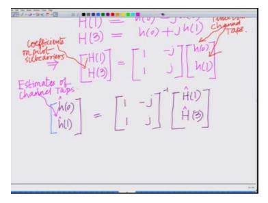
Now therefore, I can find the channel taps as the channel taps can be found simply as h 0 h 1 equals this 1 - j, this matrix inverse times H 1 H 3 and that is basically what we have. And the last step is basically to realize that we have the estimates of these channel coefficients on the pilot subcarriers, so if we use the estimates here on the left hand side also, you will get estimates.
