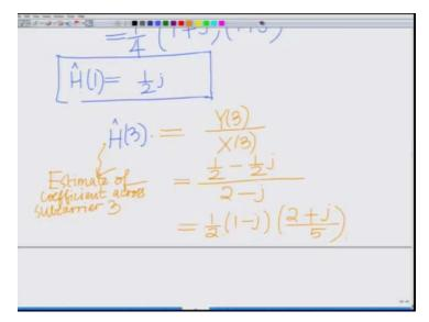
That is, estimate and this is equal to Y 3 divided by X 3 and once again from above we know both Y 3 Y 3 and X 3, that is Y 3 equals half - half j divided by X 3 that is, 2 - that is basically equal to 2 - j, which is half into 1 - j into again 2 + j divided by 5 and you can also verify this.
