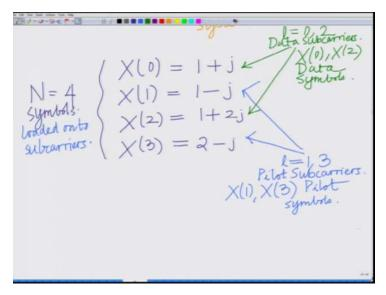
So these are N equal to 4 symbols loaded onto the subcarriers and these N equal to 4 symbols are loaded basically, that is the nomenclature that we use that these are loaded these are loaded onto the N equal to 4 symbols are loaded onto the subcarrier. However, as I said in Comb Type Pilot based channel estimation, not all the subcarriers are loaded with the pilot symbols, only a few of the subcarriers are loaded with pilot symbols.
