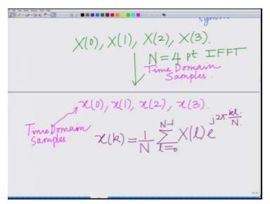
So we are going to take the N equal to 4 point IFFT Inverse Fast Fourier Transform to basically generate the time domain samples x 0, x 1, x 2, x 3, okay. So now we consider the N equal to 4 point IFFT to generate the time domain samples x 0, x 1, x 2, x 3, these are basically remember these are the time domain samples.
