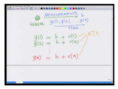
Again remember measurements, but this time it is making multiple measurements of this parameter h in time. So we have measurements y 1, y 2, y N and these are the multiple measurements being made at different time instance 1, 2 up to and so we have the measurements y 1, y 2, y N capital N measurements being made a capital N time instance.
