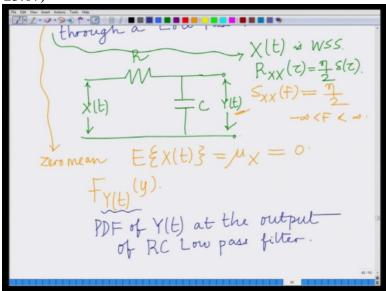
Now what we want to find in this system. So this X(t) is white Gaussian noise, 0 mean white Gaussian noise with power spectral density,  $\frac{1}{2}$ , which we are passing through this RC filter and this Y(t) is the output, what we want to find is we want to find the probability density function  $F_{Y(t)}(y)$ . So we want to find the probability density function, the PDF of Y(t) at the output, that is the noise output of your RC lowpass.
