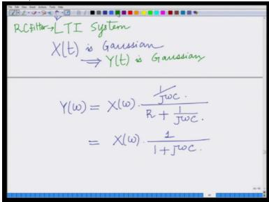
Now let us 1<sup>st</sup> find the transfer function of the system. Now most of you must be familiar with phaser analysis. So if I look at the impedance, the complex impedance of this capacitor, the complex impedance is  $\frac{1}{j\omega C}$  as a function of the circular frequency  $\omega$ .
