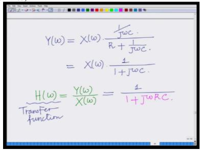
Now therefore, if a look at the transfer function. The transfer function is nothing but the ratio of the output frequency response  $Y(\omega)$  to the input frequency response  $X(\omega)$ . What is this? This is  $H(\omega)$ , which is your transfer function,
