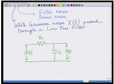
Let us consider a simple lowpass filter. Let us consider this RC lowpass filter. So the input to this lowpass filter is your random process X(t), the output is your random process Y(t). So we are saying let us consider what happens to a noise process at the receiver in a communication system when you pass it through a filter. We are assuming that this noise process X(t), which is a white Gaussian random process. Right? This is a white Gaussian random process.
