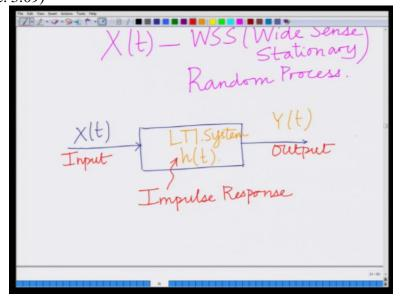
So we are saying, this wide sense stationary random process X(t) is input to a linear time invariant system with impulse response h(t) and that I want to represent that schematically over here. So I have my LTI system. This is the input to the LTI system. So, X(t) is the input to LTI system, Y(t) is the output of the LTI system. So this is my LTI system which is characterized by the impulse response h(t).
