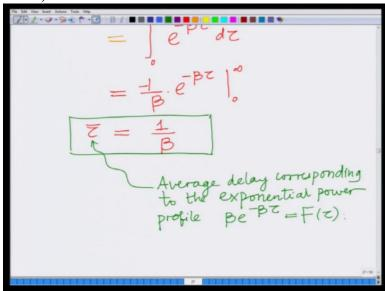
$\overline{\tau}$  is average delay corresponding to the exponential power profile  $e^{-\beta\tau}$ . So we are saying, corresponding to the exponential power profile in the multipath wireless channel where
