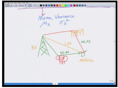
which is transmitting to the mobile. So there is a direct line of sight component, a signal which goes from the base station to the mobile. And because of reflectors, there are several scattered components. Because of obstruction such as buildings, etc in the wireless environment, there are several non line of sight components.
