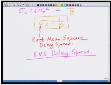
This is also known as the root mean square delay spread or the RMS delay spread of the wireless channel. This equal to 1 over  $\beta$ .
