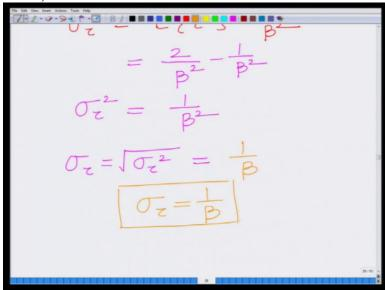
So we have the standard deviation equals 1 over  $\beta$  and this is an important parameter in wireless communication.
