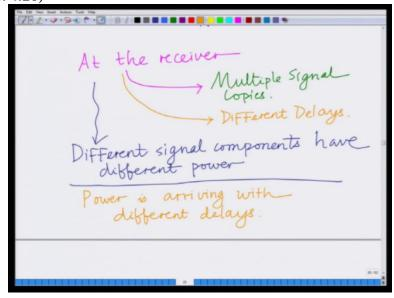
So different signal components arrive at different delays and these different signal components have different power. So basically, the power, one can say that the power is arriving with different delays.
