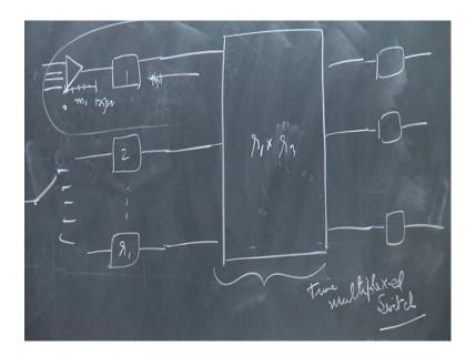
And this space switch is of, how much dimensions? r 1 by because, the r 1 inputs are there, m 2 is equal to r 1, and n 2 is equal to r 3. So, this will be r 1 by r 3 switch technically. So, there is instead of having r 2 switches I have only 1 switch only problem is, when the slot number one will come it is through some interconnection pattern, it will act like switch number 1 or middle stage, when slot 2 will come my interconnection should change.
