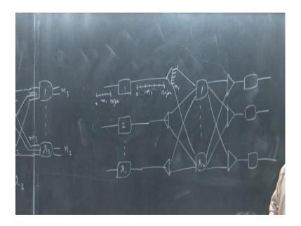
So, 125 micro second and x the n read access and n write access is 2 n. So, this is the access time, which is available for each word for read write. So, this has to be always greater than or equal to t access; which actually implies your n has to be less than equal to 125 micro second by 2 into t access. So, you require a very fast memories if you require a higher n. So, this value will if you keep as less as possible.
