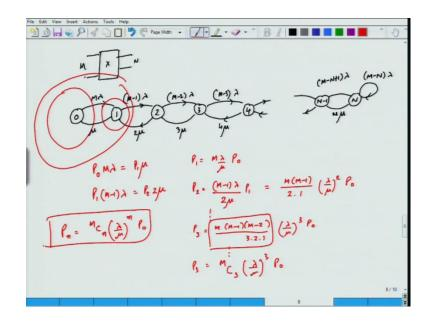
So, your m by N composite switch is going to be... So, there is no call there. So, the arrival, which can happen will happen with the rate, m lambda delta t. Remember, delta t I N is going to cancel, when I am going to have a balance equations to be built for a steady state situations. So, I need not I can actually remove delta t. In fact, earlier time the delta t cancels from both sides I need not keep it so.
