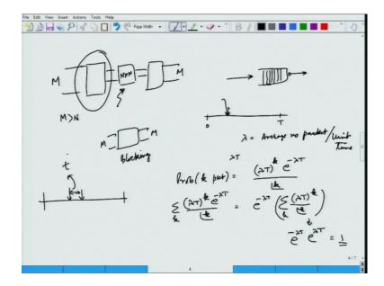
And then I actually use what we call expanded cell compressors, which basically is a special kind of a switch where large number of incoming ports are there, on one side than smaller on this side, with the assumption that, all users will not be active at any point of time. So, chances you will be blocked is very small, but because of which my hardware reduction is much drastic, which will help in deducing the call cost.
