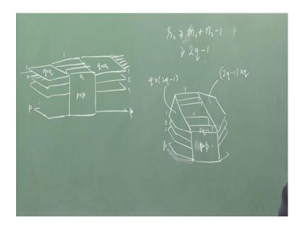
And in checked I can draw this something like this. So, this is q by q each one of them, 1 2 and so on, and you have total p switches like just put boards like this. So, there are q inputs and q ports going on, and then I can create at cross connection and so on. So, it is 1 2 q each 1 of them is p by p. So, these are q ports coming out, and here q ports going in. So, you can actually look into this kind of structure.
