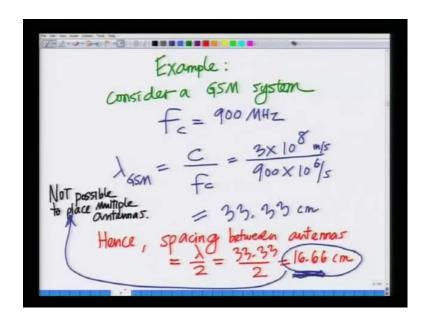
We said in a 2G GSM system 900 mega hertz lambda is 33.33 centimeters which means lambda by 2 is over 16.66 centimeters which is greater than the dimension of a cell phone. So, it is not possible to place multiple antennas on a 2G phone.
