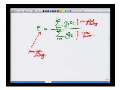
Now, I can write this as tau bar equals summation i equals 0 to 1 minus 1 That is the total number of paths g i which g i is the gain of the i th path times tau i where tau i is the delay of the i th path. It is divided by the total power which is i equals 0 to L minus 1 g i i equals 0 to L minus 1 summation g i. So, this the numerator is the weighted delay and the denominator is the total power, so this is essentially the normalized delay or this is the average.
