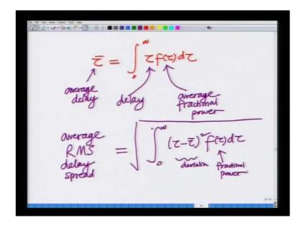
I can define the average power profile i can define the average delay tau bar as integral 0 to infinity tau f of tau d tau look at this, this is the delay weighted by the average fractional power. This is similar to computing the expectation of a random variable which is i am taking delay tau I am weighing it by the average fractional power. This is similar to what we had din in the done in the case of the discrete case where we weighed the delay with p, I remember tau.
