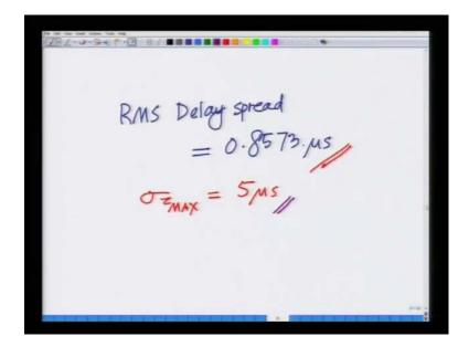
So, I will summarize this the RMS delay spread equals 0.8573 micro seconds for this wireless channel this is the RMS delay spread. Now, let us go back to the max delay spread remember we also computed the max delay spread for this channel that is 5 micro seconds. So, I will write the max delay spread side by side tau max or sigma tau max rather sigma tau max equals five micro second look at this maximum delay spread is much larger than the RMS delay spread which is only 0.85 micro seconds.
