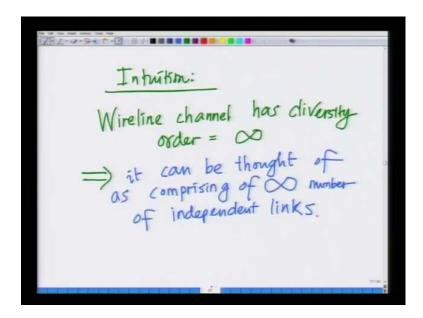
Hence, it can be thought of as comprising of an infinite number of independent links thus resulting in a very low bit error rate the diversity order of this system is infinity and we also we wrapped up the module on bit error rate diversity and wireless fading channels.
