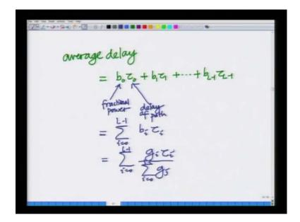
The average delay can be represented as b 0 tau 0 plus b one tau 1 plus b L minus 1 tau L minus 1 alright so look at this I am weighing by the fractional power this is b 0 is the fractional power arriving at path 0 tau 0 is the delay of the path. So, I am waving, I am weighing the delay by the power varying the delay tau 1 by the power fractional power b 1 so on and so forth.
