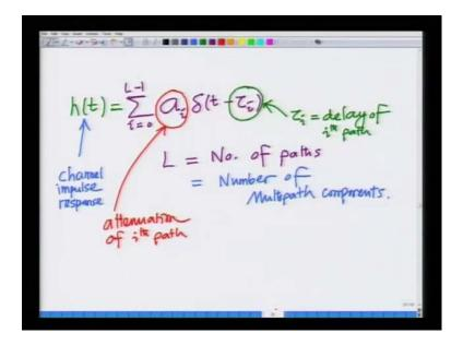
This is a multipath wireless Communication channel consisting of 1 path, each path is characterized by an attenuation a i and a delay tau i. With this let us start today's lecture which is continuing this discussion, so we said the wireless communication channel consists of 1 paths with attenuation each path having an attenuation and a delay.
