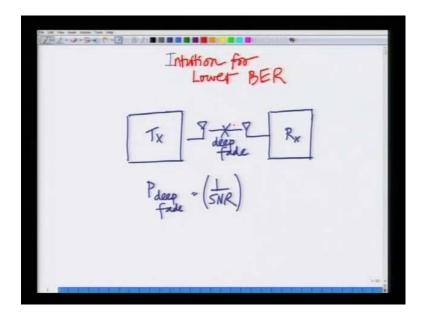
We saw why the d B r of a wireless Communication system with multiple antennas decreases as 1 over SNR power 1 where 1 is the number of receive antennas. We said the intrusion is as follows in a single antenna system I have a single link and the probability that a single link is in a deep fade is given as 1 over SN.
