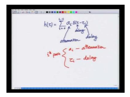
Let me now describe this again that is h of tau equals sigma i equals 0 to L minus 1 a of i delta of tau minus tau i, I have replaced that t with tau, essentially just the delay variable to indicate that this is delay variable. So, this is the delay alright so i have replaced the t by tau now you can see each path is characterized by an attenuation and a delay. So, let me write that down for the i th path a i is the attenuation factor and tau i is the delay.
