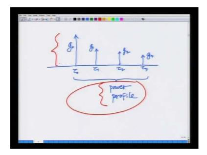
So, if I plot this profile, this arriving power profile in my fading multipath channel, it looks something like this it looks arriving path power g 0 at tau 0 second path g 1 at some delay tau 1 third path some power g 2 at delay tau 2. Then, another last path gain g three at delay tau 3, so I have four paths the 0 th path is arriving at gain 0, after some delay I have another path arriving with some power g 1 another path.
