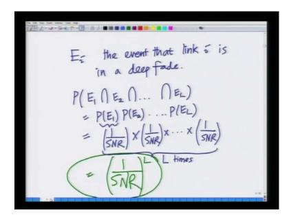
Then, the probability that the system is in a deep fade is 1 over SNR and 1 over SNR, so on so forth until 1 over SNR the whole product 1 times which is 1 over SNR power 1. These events are independent, the probability of the intersection is simply the product of the individual probabilities that is 1 over SNR power 1. Hence, the bit error rate decreases as 1
