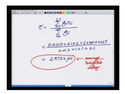
We know tau bar is simply summation i equals 0 to L minus 1 g i tau i divided by summation i equals 0 to L minus 1 g i where g i is the total received power. This is simply look at this 0.01 is the gain of the first path into 0 micro seconds which is the delay of the first path plus 0.1 which is the gain of the first path into 1 which is the delay of the first path plus 1.
