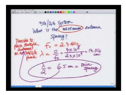
In a 3 G phone, at a carrier frequency of 2.3 Giga hertz lambda by 2 is 6.5 centimeters which is comparable to the dimensions of a phone. Hence it is possible to place multiple antennas on a 3 G phone.
