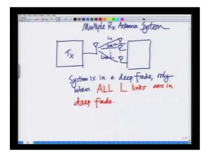
Similarly, in a multiple antenna system I have I links and the system is in a deep fade, if all the I links that is only when all the I links are in deep fade and if each of the links is independent.
