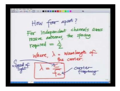
We also defined an important point, we also saw what the minimum required spacing between the antennas over the independence of the different channels to hold is. We said that the spacing is lambda equals c velocity of the electromagnetic wave v y divided by f c where f c is the carrier frequency and the spacing required is lambda over 2 where lambda is the wavelength.
