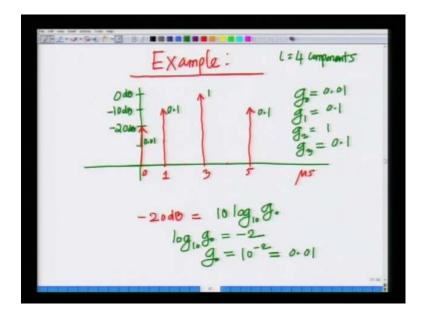
Now, let us do a simple example to reinforce this idea, so let us do an example so let me consider a channel in which alright let me consider a channel in which there are four multipath, there are four components that is I equals four components. The first component is arriving at 0, so let me draw my graph over here this is minus 10 d B and this is 0 d B. So, I have the first component which is arriving at time 0 with a gain power gain of minus 20 d B.
