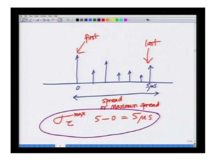
There might be a couple of paths arriving somewhere in between with some power, but the final path the last path is arriving at 5 micro seconds hence the spread or that interval over which. Hence, the spread or maximum spread is simply this interval which is the time interval between the last component, so this is the first component and this is the last component.
