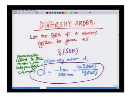
Then, we also defined another important concept in wireless communication system which is the diversity order which is defined as minus limit at high SNR. Here, as SNR tends to infinity log of probability of error as the function of SNR divided by log of SNR. We said this is approximately equal to the number of independent channels in a system.
