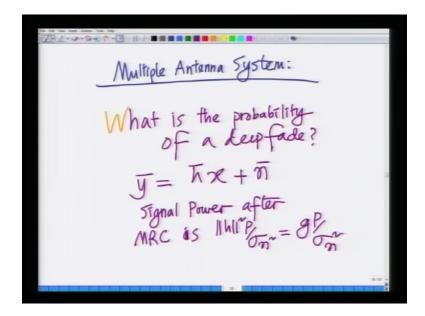
So, let us look at this multiple antenna system, let us look at this multiple antenna system and let us again ask the question that we asked before. What is the probability of a deep fade in this term in this multiple antenna system, what what is the probability of a deep fade in this multiple antenna system, what is the probability that the system is in a deep fade.
