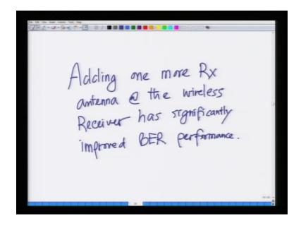
Adding one more R x antenna of the wireless system at the wireless receiver, has significantly improved bit error rate performance. So, adding one more receive antenna at the receiver in my wireless communication system, has significantly improved the bit error rate performance, and hence this scheme receive diversity is a very important technique in 3 G, 4 G wireless communication systems.
