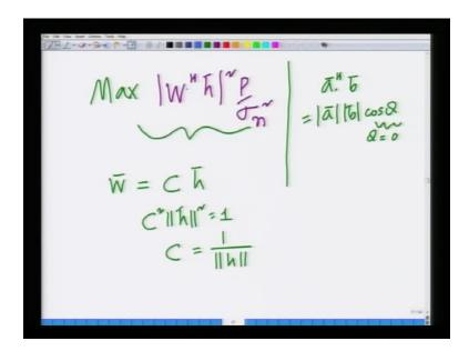
And we said we also wanted to derive that or compute that optimal vector w bar, which maximizes the SNR at the receiver and we said that can be derived by maximizing w bar Hermitian h norm square that is the vector w bar, which maximizes w bar Hermitian h bar norm square maximizes, the SNR at the receiver.
