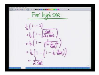
Now, let me slightly simplify this for the co case of high SNR, let me simplify for so, let me write down here for high SNR. Now, for high SNR let us consider the term half into 1 minus lambda that is half into 1 minus SNR divided by 2 plus SNR square root, which can also be written as half into 1 minus 1 over 1 plus 2 over SNR to the power of half. So, look at this, this is half into 1 minus 1 over 1 plus 2 SNR to the power of half 1 plus 2 over SNR to the power of half is in the denominator.
