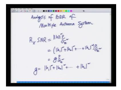
Now, let us move on to analysis of the complete analysis of the bit error rate performance of this maximal ratio combining, multiple receive antenna receiver. So, we will start our discussion today with an analysis. So, let me give the title of this that is an analysis of bit error rate of this, multiple antenna bit error rate analysis of the bit error rate of this multiple antenna system.
