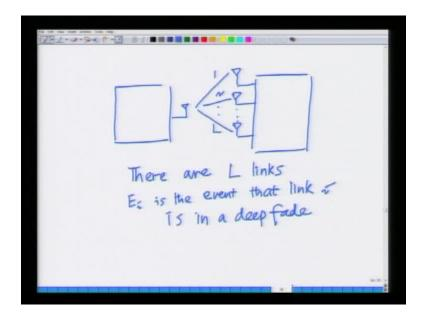
Now, let us look at what happens when we have multiple receive antennas, when we have multiple receive antennas and more specifically, we have L receive antennas there are L links in a system, with L receive antennas, there are L links between transmit antenna and first receive antenna is link 1 between transmit antenna, second receive antenna is link two so on and so forth between transmit antenna and receive antenna L is the L th link.
