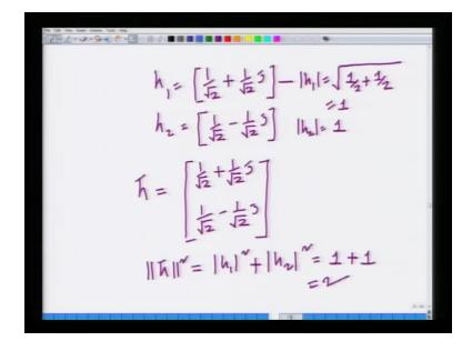
We also started with an example were we said, I have a system with two receive antennas. The fading coefficient across the first receive antenna is 1 over root 2 plus 1 over root 2 j, across the second receive antenna is 1 over root 2 minus 1 over root 2 j.
