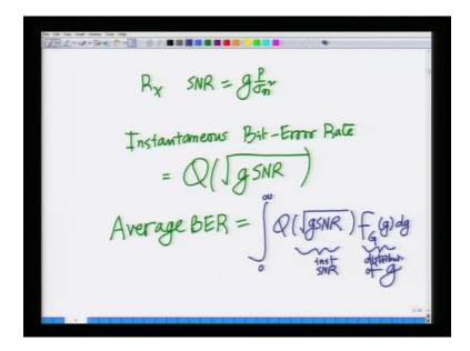
It can be shown that the distribution, f g of this gain g of this chi square random variable of 2 L degrees of freedom is shown to be given as, 1 over L minus 1 factorial times g to the power of L minus 1, e to the power of minus g. So, in other words the distribution of this gain g is f g of g, which is 1 over L minus 1 factorial times g, g to the power of L minus 1 times e to the power of minus g.
