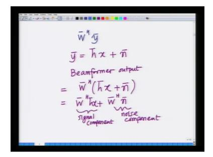
We also said that this can be succinctly represented in vector notation as w bar Hermitian times y bar, this linear combination of the signals L signals received across, the L receive antennas can be represented using vector notation as w bar Hermitian, y bar.
