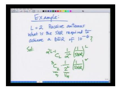
So, let us do an example let us consider the previous case where L equals 2 receive am considering the case L equals 2 receive antennas. I want to find out what is the bit error what is the SNR at which the bit error rate is 10 power minus 6 remember in the A W G N case of the digital wired or wire line communication channel case, we did the similar example we found out the signal to noise power ratio at which, the bit error rate is 10 power minus 6 is 10 power minus 6.
