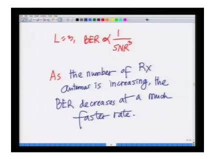
Similarly, for L equals 3 bit error rate equals 1 or is proportional to 1 over SNR cube which means, SNR cube is much larger than SNR square and SNR. So, 1 over SNR cube is much lower than 1 over SNR. Hence, the bit error rate is much lower with 3 antennas and so on and so forth. So, hence as the number of receive antennas is increasing, as the number of receive antennas increasing the exponent of SNR in the denominator is increasing right.
