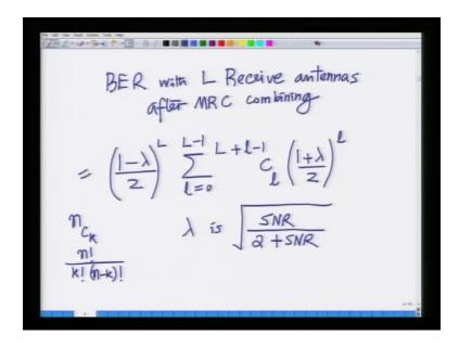
The bit error rate with L receive antennas after MRC combining the bit error rate with L receive antennas after maximal ratio of combining, we derived the optimal maximal ratio combiner, in the last lecture is given as the expression is 1 minus lambda over 2 to the power L times sigma L equals 0 to capital L minus 1 L plus L minus 1 c l 1 plus lambda over 2 to the power L.
