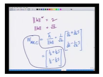
In this case, we derived the optimal maximal ratio combiner, and that we said is half plus half j and half minus half j.
