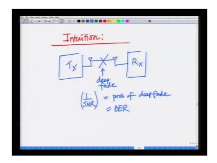
Now, intuitively why is this happening, what is the intuition, what is the intuition or what is the intuitive reason for this let us look at a system with one transmit antenna, and one receive antenna that is am saying, I have a system with one transmit antenna and one receive antenna there is only one link, we say this example earlier there is only one link the one transmit antenna, one receive antenna there is only one link, if this link was in a deep fade then the bit error rate is high.
