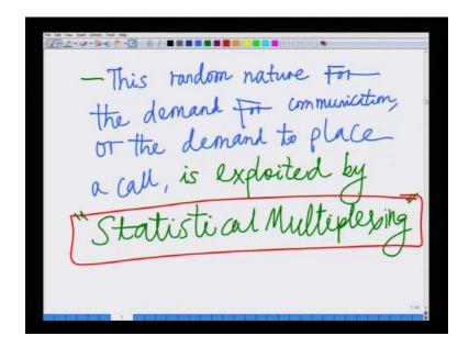
Hence, this random nature for demand for communication, or basically the demand to place a call is exploited by statistical multiplexing. This is exploited by this technique term statistical multiplexing, which essentially says that you can statistically multiplex all these users, because the placement of calls is a random event. And this statistical multiplexing may be used to support a much larger number of users with actually a very few channels, and that is
