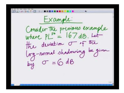
And we would also seen in the examples, in which the median path loss is 167 d B with variants of 6 d B.
