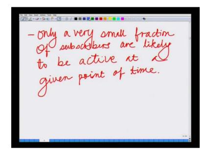
So, only a very small fraction of these users are likely to be active at any given point of time. Hence, what that means is practically, very few channels are necessary. There are n users, you do not need n channels to chater to the demands of the n users, you need only a very few channels to actually meet the demand, because only a fraction of these n users are active at any given point of time.
