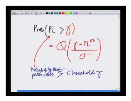
Hello, welcome to another lecture in the course on 3G 4G wireless communication systems. In the last lecture, we completed our discussion on the log normal shadowing, and we said given a median path loss P L 50, that is 50 th percentile path loss. The probability that the path loss is greater than the threshold gamma is given as Q gamma minus the 50 th percentile path loss divided by sigma, where sigma is the deviation of the log normal shadowing.
