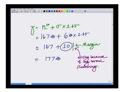
And we said the margin required for that, the margin that is that has to be accounted for this reliability factor or the transmitter is 10 d B.
