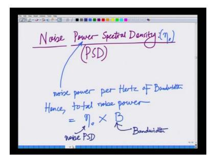
Next, we moved on to the computing noise power, receiver noise power which is essentially given by the product of the noise power spectral density eta naught times the bandwidth B.
