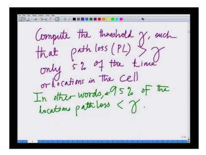
And we wanted to compute the threshold gamma such that, it exceeds threshold only 5 percent of the time, which means the reliability of 95 percent.
