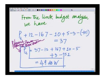
Hence, I can write from the link budget analysis we have, from the link budget analysis we have P t plus 12 minus 167 minus 10 plus 5 minus 3 minus minus 151 equals 37 db, which is the required SNR. Remember 12 is the transmit antenna gain, 167 is the median path loss, 10 is the margin and 5 is the receive antenna gain minus cabling loss, which is 3 d B minus receiver plus noise interference, which is minus 151 d B equals 37 which is the required SNR.
