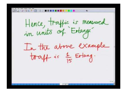
Hence, traffic is measured in units of Erlang which is denoted by the capital E, for instance in the above example the traffic is 1 by 15 erlang. All right in the above example the traffic is 1 by 15 of an Erlang now, we can compute the aggregate traffic which is the traffic given large number of users.
