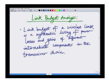
And then, we moved on to a link budget analysis, which is essentially putting all these factors together, the link budget is nothing but, the systematic listing of losses and gains in this wireless communication system which can be listed as follows.
