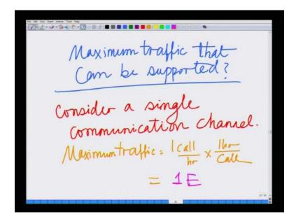
Hence, if I have 1 traffic channel, I can support N calls each for a duration of 1 by Nth of a time, hence I can support 1 erlang of traffic. Speaking of a single communication channel maximum supported traffic equals 1 call per hour into a duration of 1 hour per call which is nothing but, 1 erlang of traffic.
