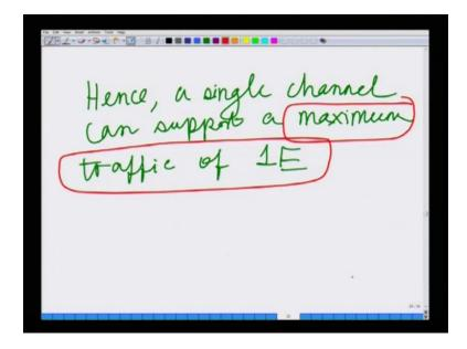
Hence, a single line, hence a single channel can support a maximum traffic of 1 erlang, hence a single channel can support a maximum traffic of 1 erlang, which means N channels. Hence,
