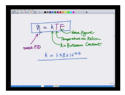
And we said the noise power spectral density eta naught can be computed as K times T times B, where K is the Boltzmann constant, T is the temperature, and F is the noise figure, all right. So, we said that eta naught can be computed as k T F all right.
