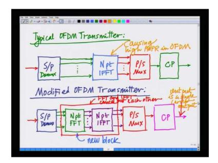
So, typical OFDM transmitter that is, how does the typical OFDM transmitter look the typical OFDM transmitter has a serial to parallel demux and followed by it has a serial to parallel demux operation followed by an N point IFFT. Then what we have is we have a parallel, we have a parallel to serial muxs operation or a multiplexing operation. Then we have the addition of the cyclic prefix as usual. Then we have the addition of the cyclic prefix this is the typical OFDM transmitter.
