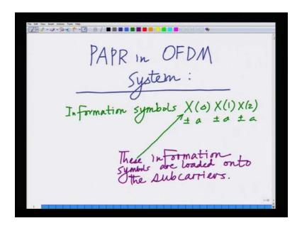
So, right now we want to start by looking at a PAPR of an OFDM system. So, consider so PAPR so PAPR in OFDM system. Now, in OFDM remember we are not transmitting the symbols as it is, but we are loading the symbols onto the subcarriers and then we are taking the IFFT of these symbols before transmitting these symbols. So, we are considering the IFFT with these symbols, all right?
