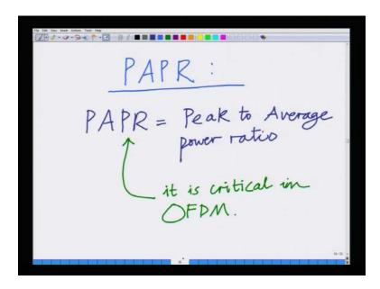
And then we had started looking at the PAPR issue that is the peak to amplitude power ratio in this OFDM system.
