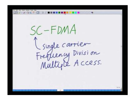
So, SC-FDMA is a variant of OFDM, it stands for single carrier frequency division multiple access.
