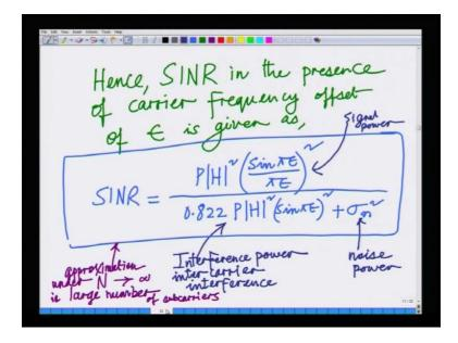
We had seen that the SINR at the receiver can be characterized as follows. That is signal power which is P magnitude H square that is the average channel gain into sine pi epsilon by pi epsilon whole square, where epsilon we said is the normalized carrier frequency offset
