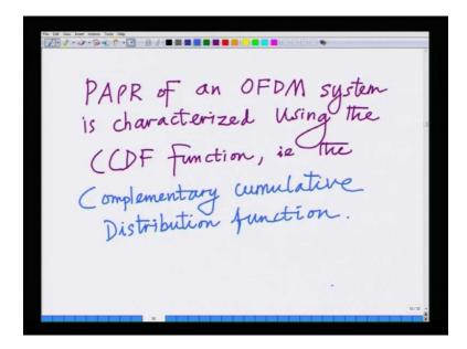
Hence, the PAPR of an OFDM characterized using the CCDF. The CCDF system is function that is the complementary cumulative distribution function that is that is the complementary cumulative distribution function. What is the complementary cumulative distribution function?
