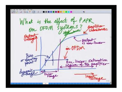
What is the problem with PAPR, what is the problem caused by PAPR? That is what we want to understand, what is the what is the effect effect of PAPR on OFDM? What is the effect of this PAPR or OFDM system? For that we have to understand a little bit about what is the characteristic of these different devices in the transceiver? If you look at specifically, if you want if you want to look at the amplifier every amplifier has what is known as an amplifier characteristic.
