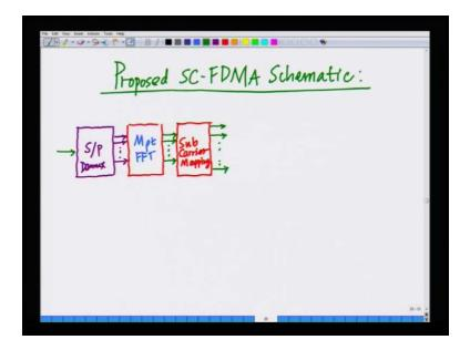
So, we want to look at the proposed SCFDMA? How does the proposed SCFDMA schematic looks as follows? That is I have a serial to parallel, again this is the demux operation that we had earlier when we form a block of symbols. Now, instead of directly doing the 50 here here, we have some M. So, we have a smaller number of symbols, so here we are going to do now an... So, we are going to take only M symbols instead of N, so here we are going to do
