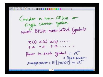
All right, we said PAPR stands for peak to amplitude power ratio and we started looking at a PAPR of a conventional single carrier system where with BPSK and amplitude level a, we said the average power across symbols is a square the peak power is a square because each symbol is plus or minus a.
