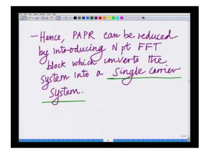
Hence, what we realize is hence PAPR can be reduced can be reduced by introducing can be reduced by introducing the N point FFT block, which converts the system FFT block, which converts the system into a. So, the PAPR can be reduced by introducing a N point FFTblock, which converts the system into a single carrier. It converts the system into a single carrier system. However, we do not want to completely move towards the single carrier system, but we want to retain the properties OFDM also.
