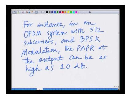
For instance and for instance in an OFDM system with about 512 subcarriers and BPSK modulation, this swing can be as high as 10 dB for instance in an OFDM system. For instance in an OFDM system with 512 subcarriers and BPSK modulation and BPSK modulation. The PAPR of the output can be as high as 10 dB for the instance in an OFDM system with 500 about five 512 subcarriers.
