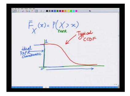
Let us consider a random variable X, the CCDF which is denoted by F bar X of F of x is simply the probability that X, which is the random variable in this case we can consider it PAPR X is greater than this value small x. That is this x can be this random variable which is
