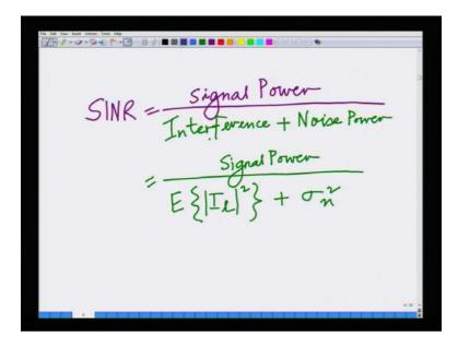
Hence, the signal to noise power ratio now can be characterized using the signal power. To the interference plus noise power since we have an SINR that is signal to interference plus noise power ratio at the receiver and last... In the last lecture we had actually developed a model to characterize this signal to interference plus noise ratio at the receiver.
