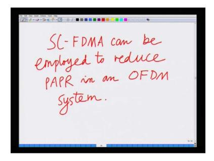
SC stands for single carrier, FDMA stands for frequency division multiple. SCFDMA stands for single carrier frequency division for multiple access and we say that an SCFDMA can be employed to combat PAPR or reduce PAPR. So, SCFDMA can be employed to reduce PAPR in an OFDM. So, SCFDMA employed to reduce PAPR in an OFDM system, all right? So, SCFDMA is that technology, which is a single carrier frequency division for multiple access technology, which is in fact employed in 4G.
