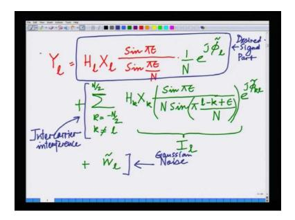
That is what we characterized in the last lecture, we had said that because of the presence of a spurious carrier frequency offset, there is a loss of orthogonality at the receiver in the OFDM system, which results in inter carrier interference that is inter sub carrier interference. Now, we have a signal component in the received signal plus an interference from the adjacent sub carriers plus the usual Gaussian noise as is shown here in this slide.
