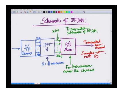
Following that, we said the schematic of an OFDM system is now simple, I do not have a bank of modulators anymore, I have a simple serial to parallel de multiplexing followed by N point IFFT, followed a parallel to serial conversion.
