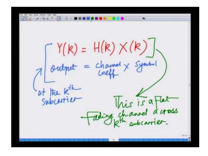
Hence, we have an elegant system in which Y k that is the received symbol across the k th subcarrier depends on H k times X k, where H k is the channel coefficient, X k is the transmitted symbol on the k th subcarrier. Hence, we have we have done is, we have converted a frequency selective fading channel into a flat fading channel across the k th subcarrier, and this is very advantages.
