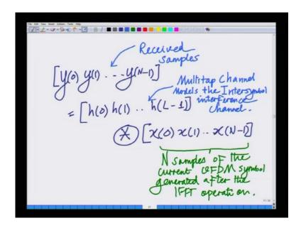
Hence, what we have is that we showed last time, that the convolution across the channel is actually converted to a circular convolution, and these are the N samples of the current OFDM symbol ok.
