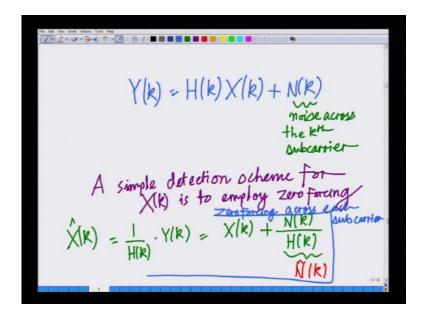
Now, I just need to mention a little bit about this detection block, what is this detection block remember across each subcarrier, we have the following relation, this is the received symbol, Y k is the received symbol, H k is the channel coefficient across the k th subcarrier, X k is the transmitted symbol, N k is nothing but, the noise across the k th subcarrier, we have not talked too much about this, but is the noise across the k th subcarrier. Now, remember X k has
