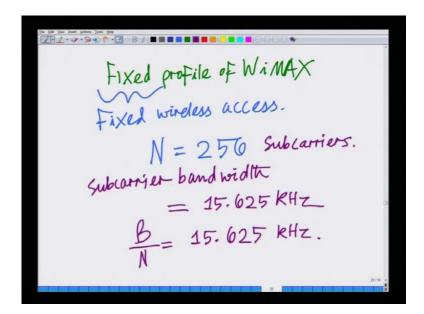
So, let us consider the fixed, so let us consider the fixed profile of WiMAX, which is essentially used for fixed. These are essentially used fixed wireless access, where wireless devices are fixed these are not mobile all right; and this profile of WiMAX has N equals 256, this profile of WiMAX is N equals 256 subcarriers; it is a 4G standard and the subcarrier bandwidth, the subcarrier bandwidth equals 15.625 KHZ.
