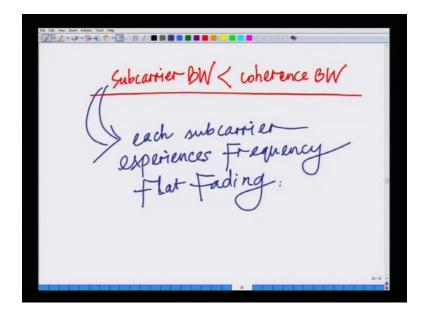
So, this implies each subcarriers experiences, each subcarrier experiences frequency flat, so by increasing N as described above, what is as it is happening is subcarrier experiences frequency selective fading. Hence, an appropriately designed OFDM system converts a frequency selective fading channel into a set of parallel fading flat fading channel across the subcarrier.
