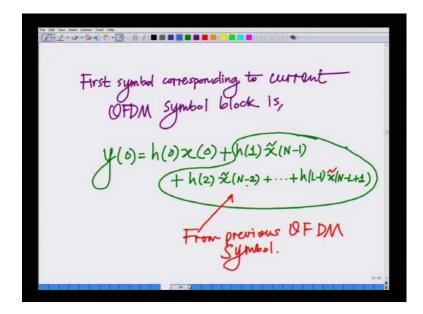
Following that, we said that the first symbol corresponding to the current OFDM symbol block, let us say we consider transmission of an OFDM. Hence, there is inter symbol interference from the previous transmitted OFDM samples all right.
