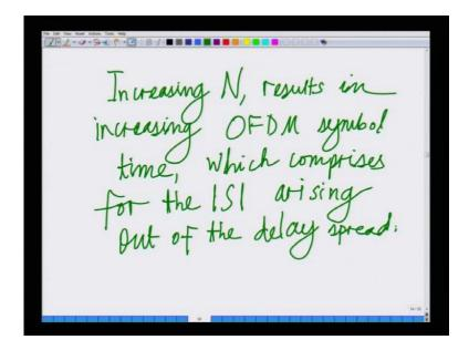
Hence, one can also think of this as N by B increasing, N by B compensate for the ISI arising out of the delay spread, hence we can also think of the increasing N results in increasing, increasing OFDM symbol time, increasing OFDM symbol time which compensates for the ISI. So, ISI becomes the progressively smaller fraction, which comprises for the, for the ISI arising out of arising out of the delay spread. However, what is the trade of an increasing N?
