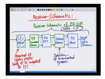
So, how does the receiver schematic corresponding this thing look like, so what is the receiver schematic? So, how does so, this I will also write, this is the transmitter schematic, so this is the transmitter, this is the transmitter schematic. And how does the corresponding receiver schematic look with the addition of the cyclic prefix, and that looks as follows.
