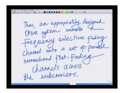
Let me, just note down this final point, thus an appropriately designed OFDM system converts, a frequency selective fading channel converts a frequency selective fading channel, with ISI converts a frequency selective channel into a set of parallel flat fading, narrowband channel converts a frequency selective fading channel into a set of parallel narrow band flat, narrowband flat fading.
