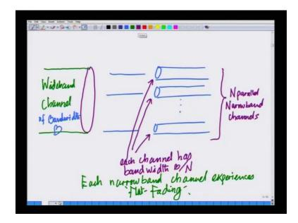
Schematically, I can expect the effect of OFDM as follows, I have a wide band channel that is let us say, this is my wideband channel, I have one wideband channel for the transmission of information, this is nothing but, also my broadband channel, this is also essentially basically the broadband channel. What I can converting this into is, I am converting this into multiple parallel flat fading channels, and each is narrowband channel.
