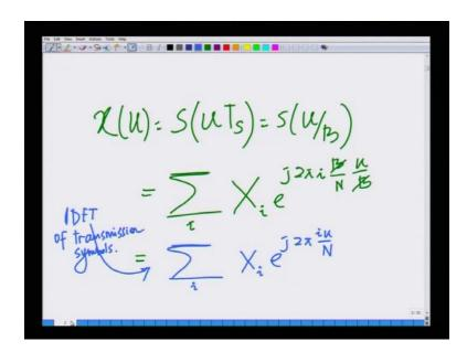
Hence, we said that the bank of modulators can be replaced by an IFFT operation.
