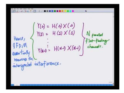
So, what we have now is that we have Y k equals H k times X k, so across each subcarrier essentially we have across the 0 th subcarrier, I can write this as Y 0 equal H 0 times X 0, I can write Y 1 equals H 1 times X 1 so on and so forth, I can write Y N 1 equals H N minus 1 times X N minus 1. So, I am converted by frequency selective channel, frequency selective channel into a set of 10 parallel flat fading channels.
