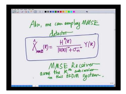
So, let me just write that equation also, also one can employ MMSE detector, and MMSE is gives you better result, and the optimal detector and MMSE detector we already know, X hat k the MMSE or X hat k MMSE is nothing but, multiply H conjugate k divided by magnitude
