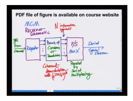
And in fact, at the receiver also the receiver oscillator has to be match in phase to the transmitter oscillator otherwise you will have phase offset and so on. So implementing this correlators and decorrelators, even one correlators, one one modulator and one demodulator is a big challenge.
