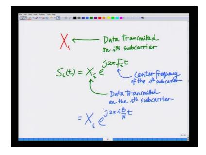
I am going to modulate the i th data stream X i onto the i th subcarrier which is given as e to the power of j 2 pi F i t. So I look at X i and I modulated onto e to the power of j 2 pi F i t; that is the i th data stream modulated onto the i th subcarrier.
