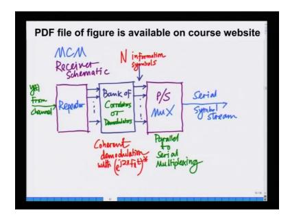
At the receiver, I have the composite signal coming from the channel, this is the composite signal s t in fact we called it also y t, because we are right now we are assuming, there are ignore neglecting the noise; just to illustrate the principles of the multi carrier modulation. So, this is y t, which is in fact equal to s t in the absence of noise.
