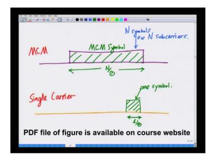
Let me just draw this pictorially in terms of picture; in a multi carrier system, I am transmitting an MCM symbols. So this is my multi carrier symbol, multi carrier modulated symbol; this has a symbol time N over B and it is transmitting N symbols on, in this I am
