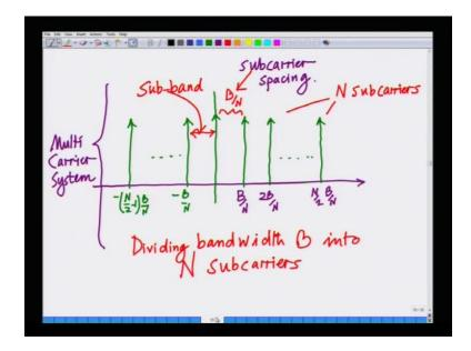
Then we also looked at, what is the essential idea behind OFDM? In OFDM, I looked at the available bandwidth B and I do not use the entire bandwidth for one carrier, but I divide that bandwidth amongst N smaller or N subcarrier. Each subcarrier comprises of a bandwidth of B over N that is each subcarrier comprises of a bandwidth; the bandwidth allocated to each subcarrier is B over N; I have N subcarrier, so I am taking a large bandwidth dividing it amongst multiple subcarriers and I also said.
