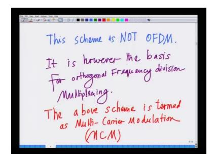
So, I want again clearly mention that this scheme is not, this is not OFDM that is the scheme that is just illustrated about is not orthogonal frequency division multiplexing. However it is the basis for orthogonal frequency division multiplexing, it is however the basis, it is however the basis for orthogonal frequency division multiplexing that is OFDM and this is has a name this scheme, that is just illustrated as a name; we are using multiple subcarriers for
