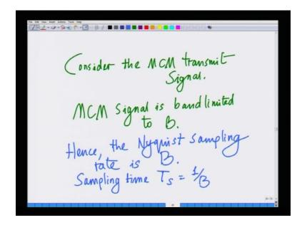
Let us consider again the MCM transmit signal, consider MCM transmit signal. Remember we have a bandwidth of B, hence this signal is limited to bandwidth of B. Hence MCM signal is, MCM signal is band limited to B. Hence I do not need to generate the time domain signal but, we have a result from sampling theory in electrical engineering which we know, if a signal is band limited to B, we can sampling it that is I am talking about the two sided bandwidth here not the one sided bandwidth.
