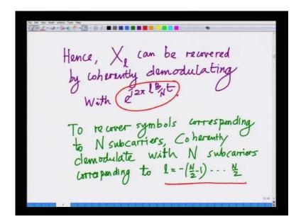
Hence, X l can be recovered by coherently; X l can be recovered by coherently demodulating with e power j 2 pi l d over N t, but coherently demodulating with that appropriate subcarrier I can, I can recover X l. So what I need at the receiver are the N demodulators e power j 2 pi l
