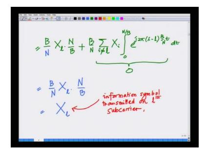
Now, the X l comes out of integration this i can write as B over l times X l into N over B plus B over N times summation i not equals l X i 0 to N over B e to the power of j 2 pi i minus l B over N t. And as we said by the previous argument, this integral 0 to N over B e power j 2 pi i minus l B over N t is in fact equal to 0 for all i not equal to l, because we are integrating over the fundamental period.
