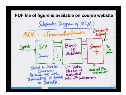
Remember let me go back to this slide, where I show the schematic of the MCM system, I need a bank of modulators conventionally. In a single carrier communication system, I need only 1 modulator and implementing that 1 modulator itself is a significantly challenging,
