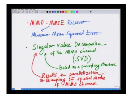
So, we also proposed a in fact, this is the MIMO LLMSE receiver, I will simply call this the MIMO MMSE receiver, where MMSE stands for Minimum Mean... So, essentially this MIMO MMSE receiver; it minimizes the mean square of error of detection at the receiver, and we also saw that it has superior properties in the sense; that it does not result in noise enhancement, because of its unique structure.
