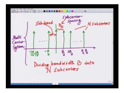
Let me, consider a system, in which I have a bandwidth of B. Again remember, I am talking about the two sided bandwidth, and what I am going to do is instead of having one single carrier, I am going to divide it into multiple carriers divided into multiple carriers at a spacing of B over N.
