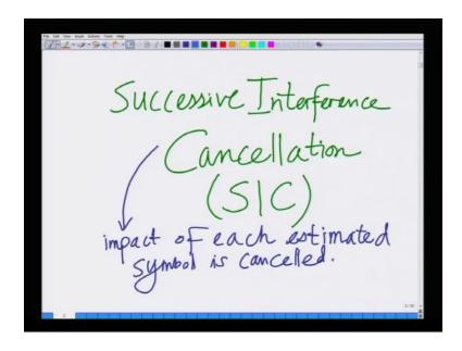
In the last lecture, we discussed the non-linear V blast receiver for MIMO communication systems; we also said that, this receiver is based on the SIC principle; that is successive interference cancellation, where are symbols are estimated and their impact is successively cancelled followed by detection of other symbols and so on. This is an iterative procedure essentially.
