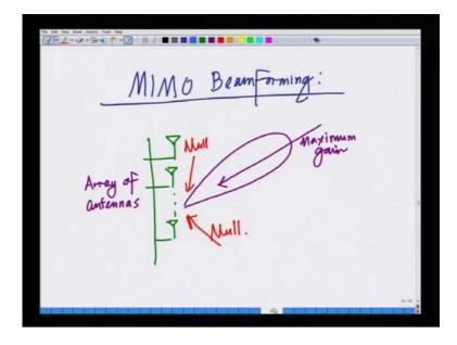
Then, we had also talked it, talked about beam forming; that is forming a beam in a MIMO communication system; that is a instead of employing all the modes, we transmit only in a certain given direction in n dimensional space, which is less beam forming.
