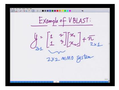
And, we had also seen an example of a V blast system of the simple V blast receiver for a 2 cross 2 MIMO system.
