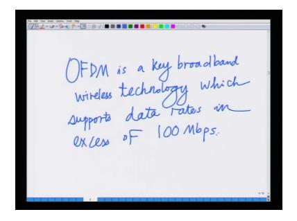
So, OFDM is a key broadband wireless technology, which supports data rates in excess of... So OFDM is a key broadband wireless technology, and it helps, it supports essentially one of the key technologies, which supports data rates in excess of 100 mbps, which is crucial and next generation broadband wireless communication systems and communication networks alright, and also further not only cellular standard, OFDM is also the basis for land standards.
