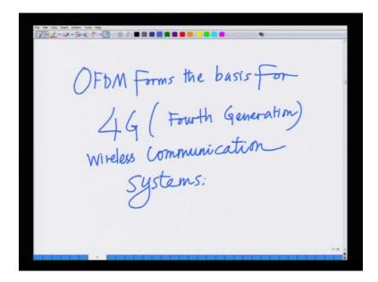
So, OFDM is very important, because OFDM forms the basis for... it forms the basis for futuristic 4G or fourth generation or 4G, which is essentially fourth generation wireless communication systems alright. So, OFDM or orthogonal frequency division multiplexing is a very important technology, revolutionary radical technology in wireless communication systems, because it is a key technology for 4G wireless communication systems.
