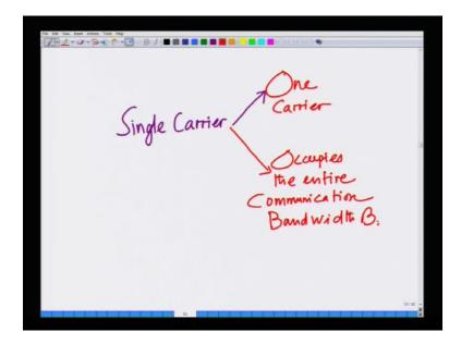
As, we have seen; this is a single carrier communication system; what it means is? There is one carrier, this is a which means; there is a unique carrier; that is one carrier and that consumes the entire bandwidth, that occupies the entire communication bandwidth. There is a single communication carrier; and that occupies, the entire communication bandwidth of B and that is the philosophy of a conventional single carrier system alright.
