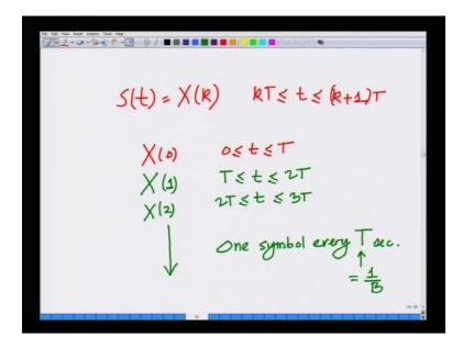
And, if you look at the transmission itself the transmission can roughly be expressed as follows as s t equals x k for k T less than equal to t less than equal to k plus one T alright for
