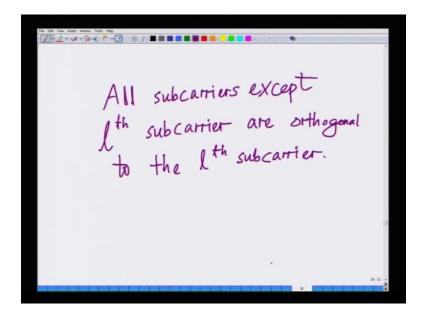
Let summarize this, here all sub carries except lth, all sub carriers except lth sub carrier all sub carriers except lth sub carrier or essentially; this results in an output of 0; they are orthogonal. Hence, I can essentially coherently demodulate by correlating with e power j 2 pi f 1 of t; that is essentially. I am multiplying by e power minus j 2 pi f 1 of t and integrating over the fundamental period, which is 0 to N over B.
