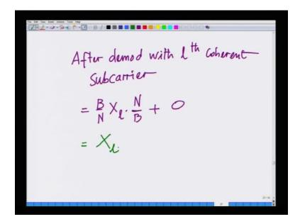
After demodulation is after demodulation in the coherent, lth after demodulation with lth coherent sub carrier, what I have is, I have this is equal to B over N into x l into the integral N over B plus rest all sub carrier gives 0, hence this results in x l.
