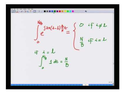
So, this integral so let me again, simplify this integral e for j 2 pi i minus l i minus l b over N t from 0 to B over N, which is N or you can write it, sum 0 to N over B; this integral e equals this integrals equals 0, if i knot equals l and this integral e equals, in fact if you look at this, if i equals l; this integral becomes 0 to N over B e for j 2 pi i minus l i equals l, since this is 0 e power j 2 e power 0 is 1.
