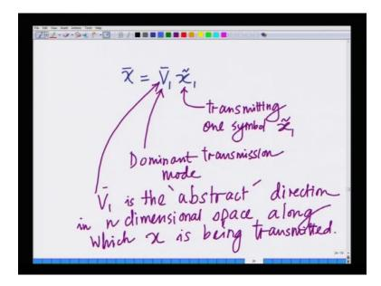
For this purpose, we said that the x bar vector can be formed as at beam in the direction of v 1 bar, where v 1 is the dominant right singular vector of the matrix H, employing was single transmitted symbol x 1 tilde.
