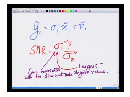
And corresponding to that, we said the received SNR was sigma 1 square P over sigma n square, so it exact. So, the gain of this channel is sigma 1 square, which extracts the dominant or which corresponds to the dominant singular mode of this MIMO channel.
