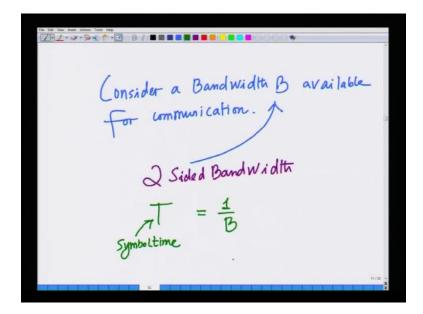
So, we can consider a band width. Let us, start by considering a band width of B; available for communication. So, consider a bandwidth B available for, when I say a bandwidth B. I am considering the two sided bandwidth, here I am considering the...I am considering the two sided bandwidth B; that is available in a traditional communication system.
