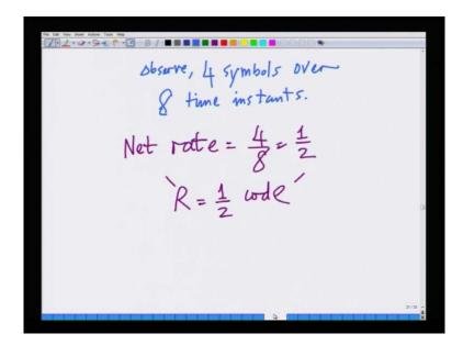
And, there was a code, which transmitted 4 symbols in 8 time instants. Hence, we said this is a rate half code. So, we had seen a rate half code orthogonal space-time block code for a 1 cross 3 MIMO system.
