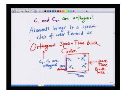
And, we also said Alamouti belongs to a unique class or space-time codes – block codes known as orthogonal space-time block codes; because orthogonal, because the different columns are orthogonal, which makes detection easier. It is a code, which spans both space and time. And it is a block code, because it involves a block of symbols; hence, it belongs to a class of codes known as orthogonal space time block codes or OSTBC.
