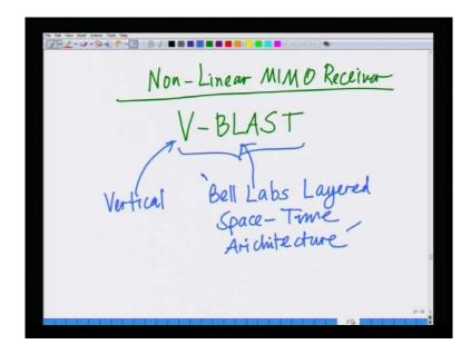
And finally, we also started our discussion on non-linear MIMO receivers with V-blast, which is the Bell Labs vertical, Bell Labs layered space-time architecture for MIMO reception. This is the point at which we left last time.
