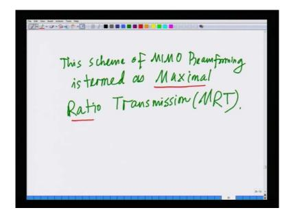
This scheme of MIMO beamforming is termed as maximal ratio transmission, that is, MRT. This scheme of transmitting along the dominant mode to obtain the gain corresponding to the largest singular value sigma 1 is termed as maximal ratio transmission – MRT. We had seen maximal ratio combining – MRC before. This is maximal ratio transmission – MRT. And the advantage of this is it results in simplistic transmission.
