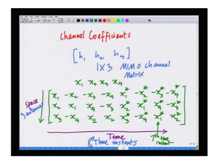
We had also seen another example of an orthogonal space-time block code for a 1 cross 3 MIMO system; that is, that has 1 receive antenna, 3 transmit antennas.
