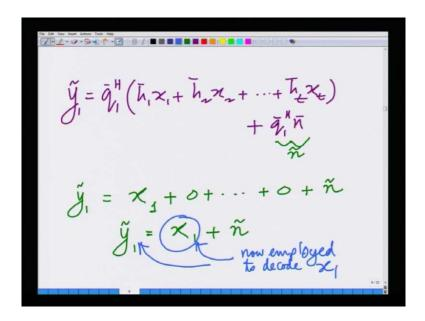
This is some noise n tilde. And at this point, I can see that, q 1 bar hermitian h 1 is 1; hence, this is one times x 1. So, y 1 tilde equals x 1 plus q 1 bar hermitian h 2 is 0 – so zero plus so on plus 0 plus some n tilde. So, now, what I have done essentially is I have induced the properties of the zero forcing receiver left multiplied by q 1 bar hermitian, which is orthogonal to h 2, h 3 until h t. And I have cancelled the interference from those streams.
