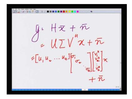
So, for instance, I have y bar equals H x bar plus n bar; that is, the MIMO system. I am going to consider the SVD of this. Remember we have looked at the singular value decomposition of this; I am going to write this as U sigma V hermitian; that is, the matrix H can be written in
