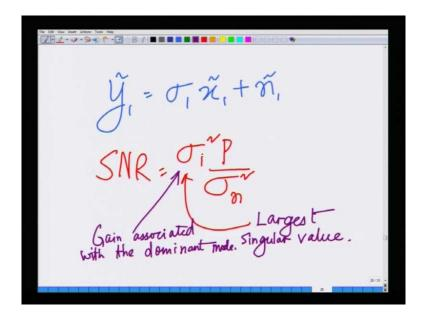
This y 1 tilde equals sigma 1 x 1 tilde plus some noise n 1 tilde. This is what I have. And the SNR associated with... SNR equals sigma 1 square P; where, P is the power in the transmitter
