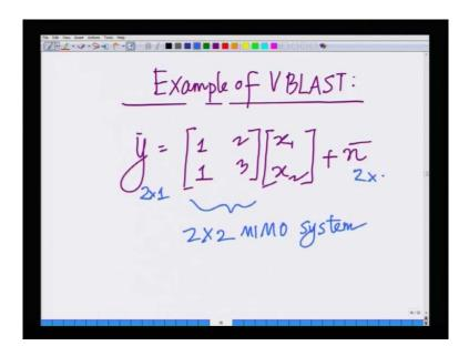
So, let us proceed to the example. I am going to consider again a 2 cross 2 MIMO system; y bar equals 1, 1, 2, 3; x 1, x 2 plus n bar. So, I am considering a 2 cross 2 MIMO system. So, this is a 2 cross 2 MIMO system. I am transmitting two symbols: x 1, x 2; receive the vector y, which is 2 cross 1 dimensional noise bar. Vector is also 2 cross 1 dimensional. You should be very familiar with this system model at this point.
