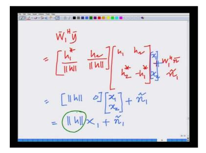
So what I am going to do is; I am going to perform w 1 Hermitian y bar. So I am going to perform w 1 Hermitian y bar which is nothing but, h 1 conjugate divided by norm h h 2 divided by norm h into h 1 h 2 or h 2 conjugate plus w 1 Hermitian n bar. I will denote this by some n 1 tilde.
