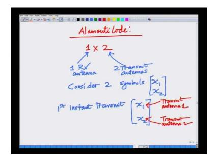
So I am going to consider a 1 cross 2 system that is, so let me illustrate the Alamouti code; it is a 1 cross 2 system, 1 receive antenna. So I am going to consider 1 cross 2 system which means, 1 receive antenna and 2 transmit it has 1 receive antenna and 2 transmit antennas. At the first instance, so we consider 2 symbols consider 2 symbols x 1 comma x 2. We consider 2 symbols x 1 comma x 2 at the first instant, we transmit first instant, we transmit the transmit vector x 1 comma x 2.
