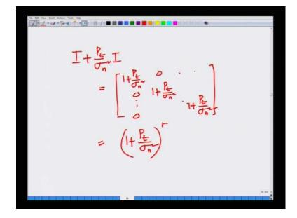
This matrix is nothing but, this matrix is nothing but, 1 plus P t over sigma n square 1 plus P t over sigma n squared 1 plus P t over sigma n squared and the off diagonal terms are all 0. Hence the determinant of this matrix is nothing but, 1 plus P t over sigma n squared to the power r and when you take log of the determinant that is nothing but, r times log 1 plus P t over sigma n squared.
