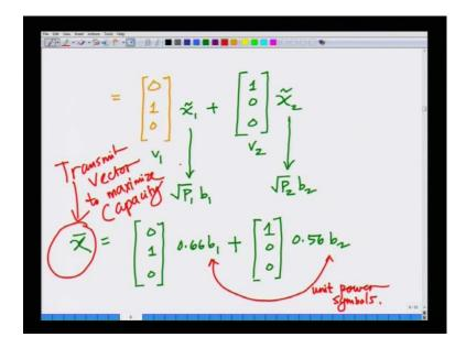
Remember these are the vectors v 1 and v 2, these are also the beam formulation remember, you cannot simply transmit any transmit vector but, you have to pre-code whatever transmit symbols are there, with this transmit with this matrix v alright. That is what we said that is what results in the decoupling and now this easy x 1 tilde is nothing but, you have to allocate power P 1 to it is. So this is square root of P 1 into b 1, where b 1 is a unit power symbol.
