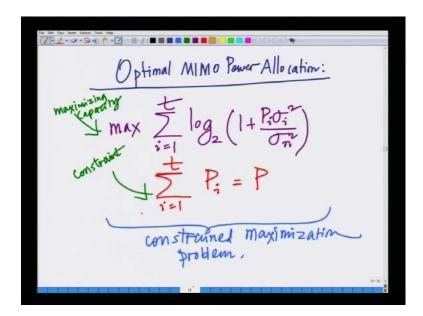
We have also said the capacity of this channel is the sum of the capacities of these t individual channels that is log 2 1 plus P i, which is P i is power allocated to ith channel sigma i square divided by sigma n square summation over the t channels. And we want to maximize this capacity such that this transmit power P 1, P 2, P t allocated to each of the t channels is limited by P which is the total transmit power.
