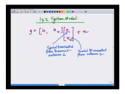
And my system model can be expressed as what is the 1 cross 2 system model; that can be expressed as the received symbol y equals h 1 h 2, which is my 1 cross 1 MIMO system times x 1 x 2 plus n. What is this x 1? x 1 is nothing but, symbol transmitted from transmit antenna 1, x 2 is symbol transmitted from transmit antenna 2 alright.
