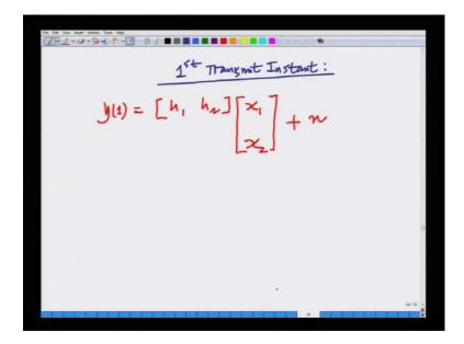
So this can be expressed as y 1 equals h 1 h 2 times x 1 x 2 plus n. This is for the first instant this is let me characterize, this is for the first transmit this is for the first transmit instant y 1 equals h 1 h 2 times x 1 x 2 plus n. Now for the second transmit instant I will do something interesting what Alamouti has proposed this is something very interesting.
