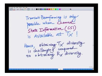
Hence, this is only possible if knowledge of the channel coefficients is available at the transmitter. Hence, transmit beam forming is only possible when channel knowledge or channel state information channel knowledge or channel state information is available at the transmitter.
