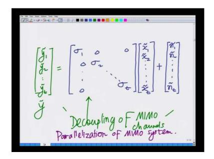
Welcome to another lecture in the course on 3G 4G wireless communication systems. In the last lecture, we employed the concept of the singular value decomposition of a MIMO channel and reduced it to a decoupled MIMO wireless channel as y tilde equals the diagonal matrix sigma times x tilde plus n tilde bar, where this is arrived at as we said by multiplying y with u Hermitian and pre-coding the transmit vector x as x equal to v times x.
