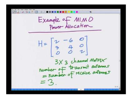
And we also started with an example of this channel matrix H 2 minus 6 0, 3 4 0, 0 0 2. We computed its singular values as follows; that is square root 52, square root 13 and 2 and corresponding to these singular values.
