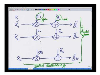
And we have also described this schematically we drew a picture we said it can be consider as t different channels with x 1 tilde transmitted as P 1 gain sigma 1 noise n 1 tilde x 2 tilde transmitted across channel with gain sigma 2 into tilde noise so on and so forth.
