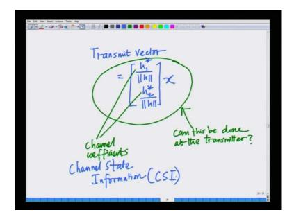
Let us go back to what we have done? We have done a transmit pre-coding where we said the transmit vector is h 1 conjugate divided by norm x h 2 conjugate divided by norm h times x. Now can this be done at the transmitter? Can this operation be done? Or can this operation be done at the transmitter? Is the question which want to ask ourselves.
