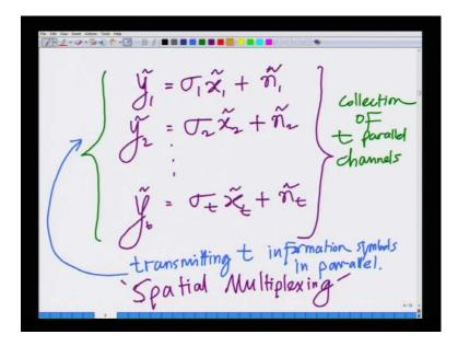
And we said as a result I have y 1 tilde equals sigma 1 x 1 tilde plus n 1 tilde y 2 tilde equals sigma 2 x 2 tilde plus n 2 tilde so on hence so forth. So this MIMO channel has become decoupled into t parallel channels, this is also as we said spatial multiplexing.
