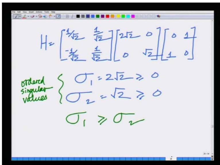
$$H = \begin{bmatrix} \frac{1}{\sqrt{2}} & \frac{1}{\sqrt{2}} \\ -\frac{1}{\sqrt{2}} & \frac{1}{\sqrt{2}} \end{bmatrix} \begin{bmatrix} 2\sqrt{2} & 0 \\ 0 & \sqrt{2} \end{bmatrix} \begin{bmatrix} 0 & 1 \\ 1 & 0 \end{bmatrix}$$
