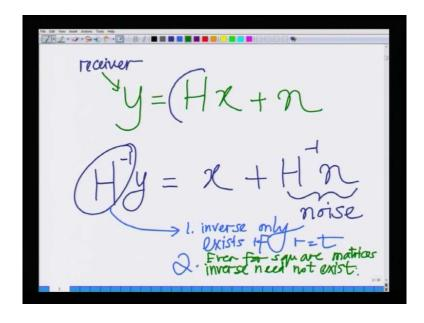
So, the MIMO system model can be described as y equal H x plus n as we have seen x is the transmit symbol vector, y is the receive symbol vector. Now, one simple receiver to do in this case is at the receiver once I receive y, so this is at the receiver I have y. So, at the receiver I will invert the channel matrix I will perform H inverse y that is equal to H inverse times h which is identity times x hence this is x plus H inverse of n.
