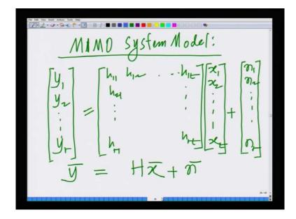
And we saw that this can be represented using a matrix notation as y 1, y 2, y r which are the r symbols received at the r. Receive antennas can be represented as an r cross t matrix which is the channel matrix h times x 1, x 2, x t, which is the t dimensional transmit vector that is
