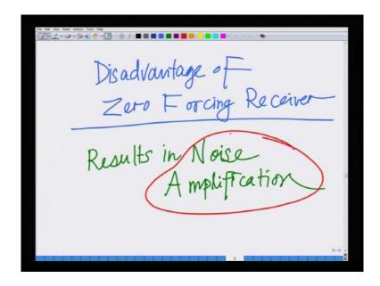
So, let us write the disadvantage zero forcing receiver, the disadvantage of zero forcing are it results in noise it results in noise amplification that is the disadvantage of MIMO zero forcing receiver. Now, low value of the channel when channel is close to zero, in the matrix sense, we cannot quantify it right now, because it does not because there is no sense in saying a matrix is close to zero.
