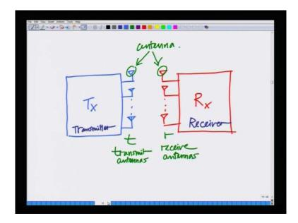
And MIMO system can be simply represented as having multiple antennas at the transmitter and the receiver that is I take a conventional system, which only has a single antenna at the transmitter, and single antenna at the receiver. A MIMO system has multiple antennas at the transmitter and multiple antennas at the receiver.
