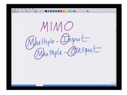
And then we had moved on to a new module namely MIMO which is its MIMO stands for Multiple Input Multiple Output communication systems.
