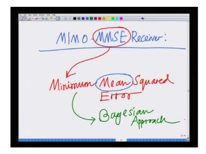
So, we are going to look at another alternative receiver which is robust to noise enhancement or which avoid the problem of noise enhancement that known that is known as the MIMO MMSE this is known as the MIMO MMSE receiver.
