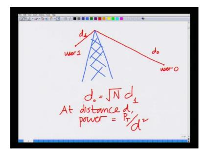
So, I am considering a base station. Now, in this base station there is user user 0, who is at a distance d 0 and there is a user 1 who is closer to the base station at distance d 1, all right? So, user 1 is closer to the base station compared to user 0, such that d 0 equals square root of N times d 1. Let us consider a situation where d 0 square root of N times d N. We know square root of N is the length of the CDMA spreading sequence.
