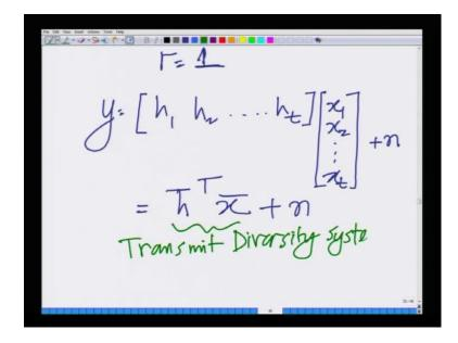
Let us consider the other special case, which is t equals 1, which is r equals , and certain number of transmit antennas. In that case we have y equals h 1, so we are considering the case where number of receive antennas r equals 1, we have not seen this case before and y
