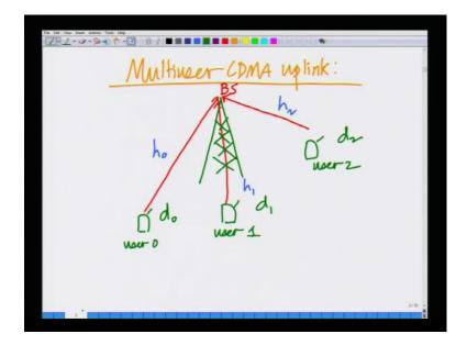
We also looked at the CDMA uplink situation which is shown here. However, uplink is slightly different from the downlink, because in the uplink the signal corresponding to different users traverse different channels and add up at the base station. Hence, this situation is slightly different from the downlink.
