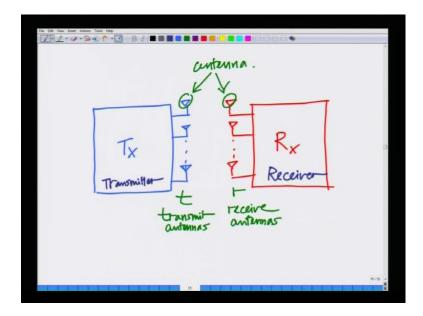
So, let me describe it schematically, let me draw a simple schematic diagram of that. I have a transmitter block and previously I had 1 antenna. Now, I have multiple antennas. Similarly, I have a receiver block, this I will abbreviate as R x and I have multiple antennas. Each of these triangular elements, each of this represents an antenna and the transmit block has multiple antennas. This is receiver block has multiple antennas, I will call the number of transmit antennas as t's.
