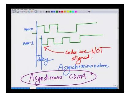
However, there is another challenge in uplink. Now, because different users are at different distances that is what we said because different users are different distances hence the propagation delays for the different signals are different. Hence, the signals at base station are asynchronous; that is if you look their edges they are not synchronized.
