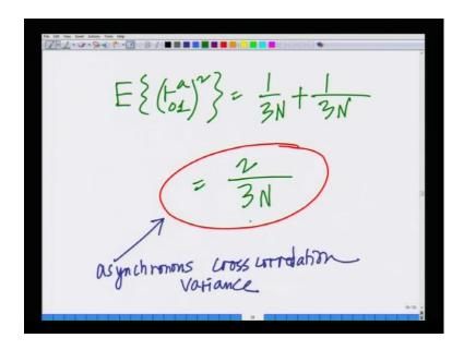
And to analyze this situation, we have to derive the asynchronous cross correlation between the sequences or the asynchronous the (( )) variance, the asynchronous interference. We said the variance of asynchronous interference is two-thirds over N, this also falls as 1 over N,0 in fact it is less than the synchronous interference because of more randomness it is two-thirds N.
