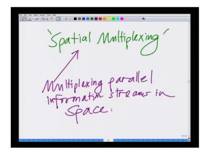
So, this is known as spatial multiplexing, which literally means multiplexing parallel information streams, multiplexing parallel information streams in space, which is essentially multiplexing these information streams in space. So, this is known as spatial multiplex and that results in a tremendous increase in the data rate, which is a unique aspect of MIMO systems.
