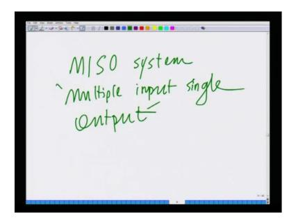
Also in the context of transmit diversity is known as MISO that is MISO system, which is multiple input single output. This is known as a MISO system, which is essentially have multiple input single output system. So, in the context of MIMO, we have two special cases when t equals 1, we know, know it as a, we term it as a SIMO system. That is single input multiple output when r equals one we term it as a MISO system, which is multiple input single output.
