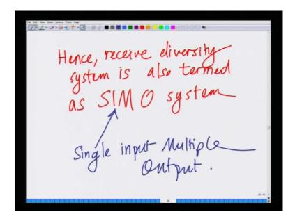
Hence, this is single input multiple output hence this is also known as the SIMO, SIMO or a single input multiple output system. Hence in diversity system is also termed as SIMO system where SIMO stands for single input multiple output SIMO also stands for single input multiple output this is termed as a SIMO system.
