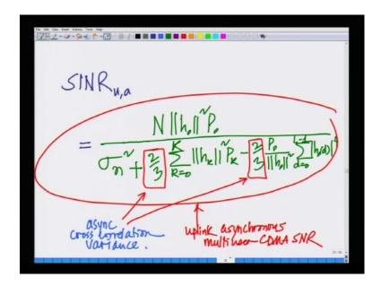
Then we simply derived the asynchronous uplink multi user SNR as N norm h square P naught, accept that the multi user and multi path interference are replaced by a factor 2 over 3. That is the only difference between the synchronous and the asynchronous link that is the power the variance of the multi user interference is reduced by a factor two-thirds that is raising because of the asynchronous nature.
