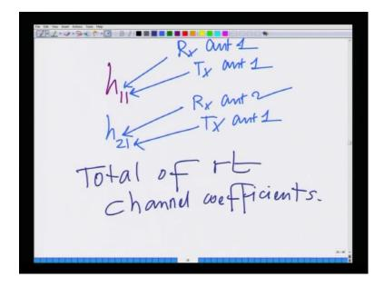
In fact if you look at h 1 1 that is transmit antenna 1, that is transmit antenna 1 and that is receive antenna 1. h 2 1 is I am sorry this has to be the other way round, this is R x antenna 1 and T x antenna 1. h 2 1 is between R x antenna 2 and T x antenna 1. Hence, between each
