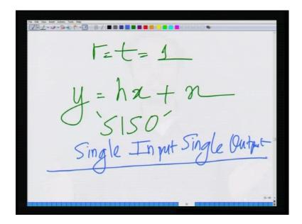
Now, obviously the next question is a special case what happens when r equals t equals 1? When r equals t equals 1, we have the traditional scalar fading coefficient channel, which is y equals h x plus n. This is naturally termed as a SISO channel, which stands for single input this naturally stands for single input, single ouput. That is the traditional one transmit antenna of one receive antenna system is also termed as a SISO system, which is single input single output system.
