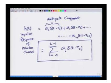
We said that the wireless communication system can be represented or each path of the system can be represented by an attenuation a i belonging to the ith path and a delay tau i belonging to the ith path. So, if there are L minus or if there are L paths indexed 0, 1 up to L
