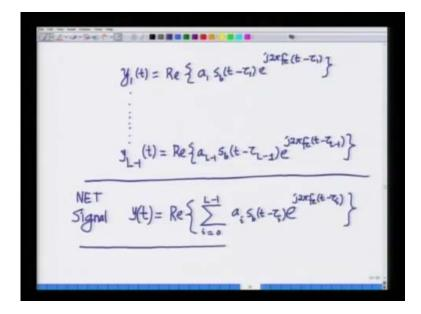
The received signal corresponding to path one is real part of a 1 s b t minus tau 1 e power j 2 pi f c t minus tau 1. This is essentially the transmitted signal attenuated by a 1 and delayed by tau 1 and so on and so forth until the signal corresponding to the L minus 1 th path is
