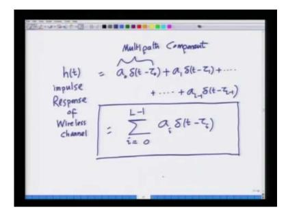
We started by trying to characterize or trying to model or develop a mathematical model for this wireless communication system as a linear time invariant system.
