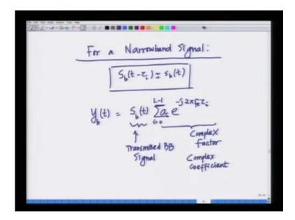
In case of a narrow band signal for a narrow band for a narrow band signal, a simplifying assumption that can be made is s b of t minus tau i is approximately equal to s b of t. What does this mean? This means that the base band signal for a different delays tau i is approximately equal to s b of t. The delay is in significant, that the delay does not cause significant distortion in the received signal, because its maximum frequency component f m is limited.
