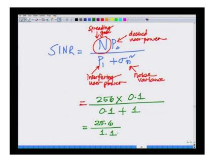
Now, we know that the signal to interference plus noise ratio SINR in a CDMA system is nothing but N times P 0 divided by P 1 plus sigma n square, this N this is the spreading gain,
