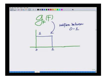
So, F is random and this fraction F is uniformly, so if I were to draw the distribution, let me denote the distribution of F by g F or the probability density function of F by g F of F, this distribution function is nothing but this is the uniform distribution. That is uniform between 0 to 1, this is F the random variable as a fraction, the delay as a fraction of the chip time which is uniformly distributed between 0 to 1.
