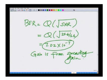
And we said the bit error rate is nothing but the BER is nothing but Q square root of SNR equals Q square root of 25.6 divided by 1.1 which is 7.02 into 10 power minus 7. Hence, we can see that at a power of minus 10 d B itself I am able to achieve a very low bit error rate of 7.02 into 10 to power minus 7. If you look at an AWGN channel we know that the power or SNR required for bit error rate of 10 to power minus 6 is roughly 13.6 dB.
