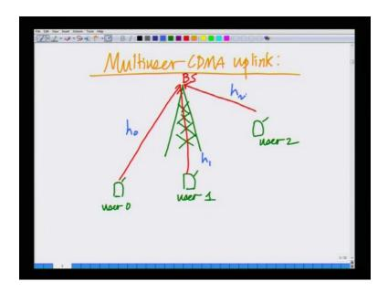
So, let us move on the multi user CDMA uplink scenario where I want to again draw a similar schematic diagram. I have a base station and there are different mobile users that is user 1 or that is user 0, user 1, user 2. Now, each user is transmitting to the base station. This is the base station; each user is transmitting to the base station. How about the direction of transmission is towards the base station, previously in the downlink base station is transmitting to the different users.
