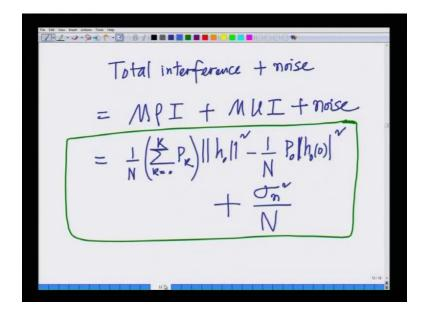
And finally, we put the multi path interference, the multi user interference and the noise together to derive the total interference that is the multi path interference plus multi user interference plus the noise power to derive the total interference plus noise ratio.
