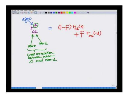
So, r 0 1 of a asynchronous can be written as 1 minus F that is 1 minus the fraction times r 0, 1 of 0 plus F times r 0 1 of minus 1. So, let me explain this as the fraction as this delay varies as a fraction of the chip time as it varies between 0 and 1. This correlation is 1 minus F times r 0 0 r 0 1 shifted, that is no shift, that is this part correlates with C 1 with no shift or the shift corresponding to 0.
