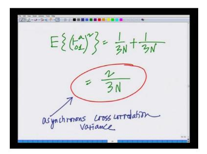
Hence, I can now write the power in the asynchronous term as expected r 0 1 asynchronous square is one-third of N plus one-third of N is nothing but two-thirds of N. This is the asynchronous cross correlation variance. This is an important quantity. This is nothing but the
