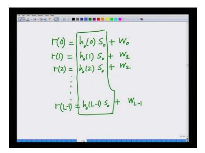
Now, we can write the signal to interference plus noise ratio. However, we also said that this is only corresponds to de correlating with respect to one path that is the zero th path. We can do it similar thing at the first path similar to what we did in a rake receiver, we can also latch on to the path, because remember, we can extract the different components. So if we de
