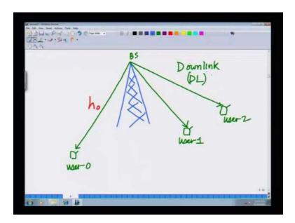
The base station, the base station is multiplying the signal corresponding to each user S 0 with code 0 S 1 with code 1 S so on so forth. S K with code k. Combining this and transmitting it, the aggregate signal on the downlink. Then we started looking at how do you process the
