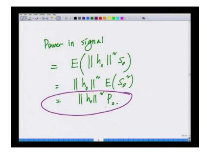
So, the power in signal is nothing but expected magnitude h 0 times S of 0. That is what we already seen before this is norm h 0 square times expected S 0 square that is norm h 0 square times p of 0. That is the power times the power in the channel. What we have seen many times before, this is what we have seen in the case of maximal ratio combiner in the rake receiver and so on. This is nothing but you coherently combining, so extracting the power multiplied by the total power in the channel.
