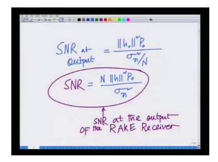
Hence, the SNR at the receiver at the rake receiver is nor h square times p o not by sigma n square, where there norm h square remember which is similar to the maximal ration combining. It represents the diversity of the rake receiver.
