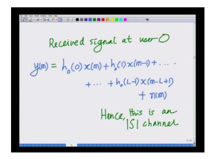
Hence, the output of this multi tap channel the received signal output of this multi tap channel, which is the received signal at user 0 through this channel h 0 is nothing but the channel h naught is nothing but h naught of 0 times x of m. This is the composite signal plus h naught of 1 times x m minus 1 plus h naught of 2 times x m minus 2 plus, so on up to h naught of 1 minus 1 x m minus 1 plus 1.
