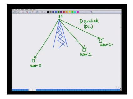
The down link scenario is nothing but where the base station where the base station is transmitting to several mobile users. So, this is the base station it is transmitting to several mobile users direction of transmission is from base station to the user, all right? So, this is the direction of transmission this is down link or d l scenario, where base station is transmitting to several mobile users. Let me call this user 0, user 1, user 2 and so on.
