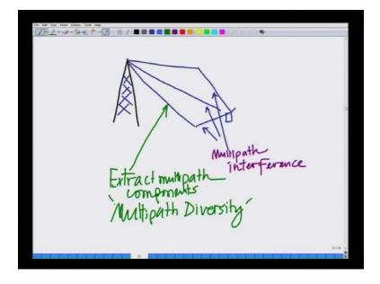
For instance if you remember what we said earlier, we said that if there is a base station in a wireless system, then there are multiple paths through which the signal reaches the user. Now, these paths can add up either constructively or destructively. Hence, they can cause constructive interference or destructive interference at the user. So, that was not it was not left to the users choice to decide whether these paths add up constructively or destructively.
