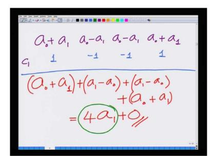
Hence, at user 0 I am correlating with his code which is c 0 and able to recover the symbol a 0 at user 1, I am correlating with his code which is c 1 and I am able to recover his symbol a 1. So, by correlating with the different codes corresponding to the different users, I am able to recover the signal both of user 0 and of user 1, hence over the common channel at the same
