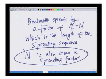
These are also hence known as spreading codes codes c 0 c 1 as we have seen they result in spreading the bandwidth of the signal, hence these are also known as spreading code. And finally, one factor that you can assume is the bandwidth increases or bandwidth spreads by a factor of 4 equals N, which is the length of the spreading sequence which is the length of the spreading sequence.
