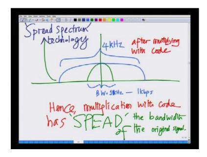
Now, I have a bandwidth which is much larger, which is 4 kilo hertz. So, remember so after this is after multiplying with code. So, before I multiply with my code the bandwidth required is 1 kilo hertz after I have multiplied with the code. The bandwidth is to 4 kilo hertz. Hence, the multiplying with the code has spread the bandwidth of the signal. Hence, this is the key word. Hence, multiplication with code has spread remember the original bandwidth which is small.
