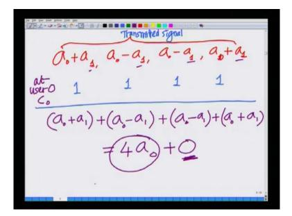
So, finally, let me write that down again what is transmitted is a 0 plus a 1, a 0 minus a 1, a 0 minus a 1, a 0 plus a 1 this is what is transmitted this is the transmitted this is the transmitted signal. So, I am taking those symbols corresponding information symbols corresponding to the user 0 and user 1. I am multiplying them with their spreading codes, I am adding these
