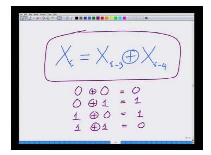
So, let me clearly illustrate this operation X i is equal to X i minus 3 combined or XOR with X i minus 4. So, the key equation that is the key equation in this linear feedback shift register architecture, that is illustrated here is the feedback path the combining in feedback path and we are saying that is generated as X i is X i minus 3 linearly combined or combined with X i minus 4. So, the equation of the feedback register is X i equals X i minus 3 X or with X i minus 4.
