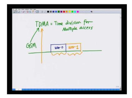
There are different ways to do it first one as we said, one way is we said is through time division for multiple access and you should be familiar that TDMA is used in GSM technology, which is the basis for all the second generation mobile phones.
