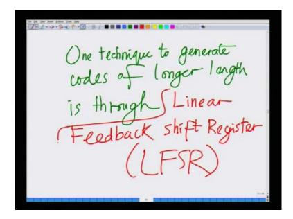
So, let me write that down one technique to generate codes of longer length is through what is known as a linear feedback shift registers. So, one so this is also abbreviated as LFSR where L stands for linear, F stands for feedback, S stands for shift and R stands for register. So, one technique to generate such sequences is through linear feedback shift registers.
