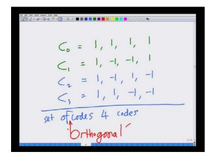
So, this is important so this terminology is important to keep in mind that it will also known as the spreading gain. Now, let us look at other such spreading codes of length N equals 4 we have looked at two codes one is c 0, which is 1 comma 1 comma 1 comma 1. We have also looked at c 1, which is 1 comma minus 1 comma minus 1 comma 1 there are two other such spreading codes one is c 2, which is 1 comma minus 1 comma 1 comma minus 1 and c 3, which is 1 comma 1 comma minus 1 comma minus 1.
