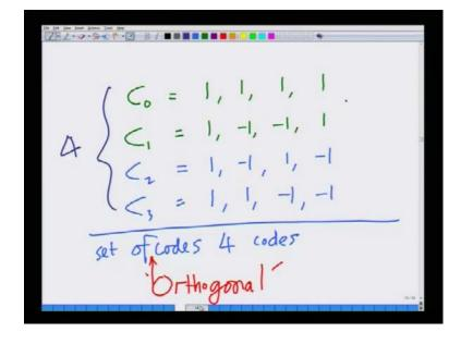
So, the number of users that can multiplex this common channel is nothing but, the number of orthogonal codes.
