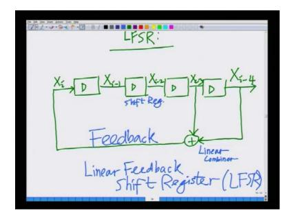
Let us, look in more detail at the structure of a linear feedback shift register as a name imply, I will first start with a sequence of registers. So, let me consider a sequence of four shift registers registers are nothing but, delay elements I will start with a sequence of four delay
