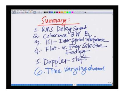
These topics included describing or characterizing the wireless channel namely with parameters such as RMS delay spread, the coherence bandwidth B c of the channel, ISI or the inter symbol interference, flat versus frequency selecting fading wireless channels, the Doppler's shift of a wireless channel, which results in a time varying wireless channel. Remember we said that mobility or Doppler shift results in a time varying wireless channel.
