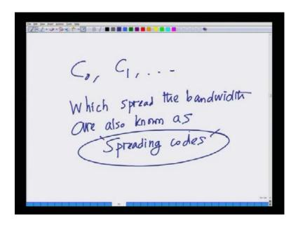
And this code which results in spreading the bandwidth is also known as the spreading code, which spreads the bandwidth is also known as code c 0 comma c 1, which spread the bandwidth are also known as spreading.
