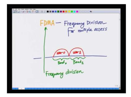
Another technology which is even before TDMA is what is known as F D MA or this also stands for frequency division for multiple access, in which instead of dividing signals in time. What I am doing is I am allocating separate frequency bands for user 0 another frequency bands for user 1. So, I am allocating band 0 for user 0 and allocating band 1 for user 1.
