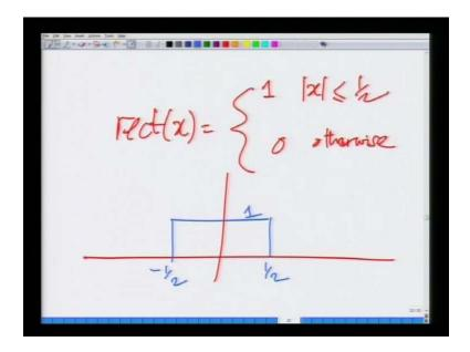
The rect function is given as follows, the rectangular x equals 1 is mod x less then equal to half 0, otherwise so the rectangular function looks as follow that is simply between minus half and half it is 1, and this is how the rectangular function looks.
