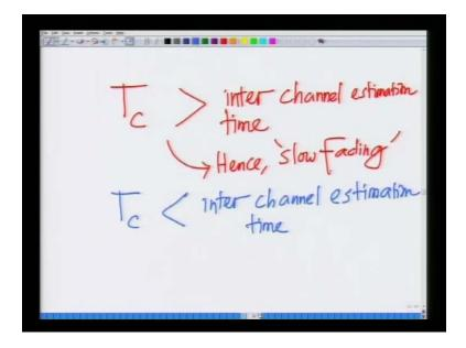
Roughly speaking a channel if T c, the coherence time is greater than the interval, successive intervals of carrying out channel estimation is, is greater than the inter channel estimation time, that is coherence time is greater than that time interval between two channel estimation
