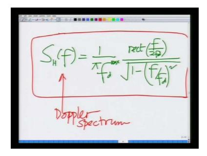
So, let we write that down that is a S H of F is nothing but, 1 over pi F d max rect, that is the rectangular function F over 2 F d divided by 1 over square root of 1 minus F over F d square. Now, we have derived the Doppler's spectrum, this is what this is the Doppler spectrum, and we are saying that is the Doppler, that is Fourier transform of the correlation function, which is in our case is the Bessel function, which can be written as 1 over pi F d rect F over F 2 F d 1 minus F over F d.
