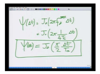
So, this is J 0, so psi of delta t is J 0 2 pi F d max of delta t, this can also be written as j 0 2 pi, remember 1 over 4 d, 1 over 4 t coherence that is 1 over 4 times coherence time is F d max, so F d max I will write as 1 over 4 T c times delta t I can also write this as J 0 pi over 2 delta t over T c. So, this coherence time or this correlation function can also be expressed J 0 pi over 2 delta t over T c that is correlation, at the channel delta t away.
