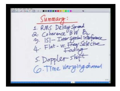
So, list of topics that is covered, so let me write the summary, in summary the list of topics that we are covered is first, the RMS delay spared, we said this the interval over which the signal power is arriving. We covered concept of coherence bandwidth, which is B c, we have covered ISI which is inter symbol interference, we have covered frequency we said that, if the delay spared is greater than the symbol time it results inter symbol interferences.
