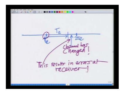
Let me draw this pictorially I have estimated the channel that is, this is a this is the time at which the channel is estimated my next channel estimation time is t e plus t e 2 t e, but coherence time is only this much which is T c, which is less than the inter channel estimation time, which means by the time I get here the channel has changed. So, if the channel if the coherence time that is the time for which the channel is constant is less than the inter channel estimation time.
