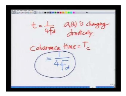
And finally, we said the time of significant change of the channel is t equals 1 by 4 F d, where F d is the Doppler frequency. The t for change is 1 over 4 F d, which is T c the coherence time, which is that interval of time over which the channel is approximately constant. That is the channel is changing, it is changing from time to time but we can assume that it is approximately constant over one coherence time interval, which corresponds to 1 over 4 F d.
