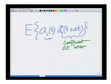
Now, what I going to compute is I want to compute the time correlation of this channel as follows, I will compute the quantity expected a i t a i conjugate t plus delta t, that is I am taking a i of t that is at a given time I am looking at the channel coefficient of I th path, I am computing its correlation with a i conjugate t plus delta t, which is the coefficient delta t later.
