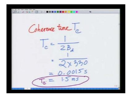
Hence, the coherence time T c, T c equals 1 over 2 B d equals 1 over 2 into 330 hertz, this is also essentially 0.0015 seconds, or I can write the same thing as 1.5 mille seconds.
