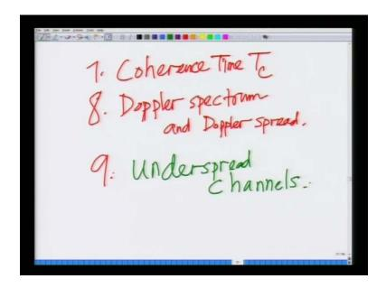
Hence what becomes important is what we considered next is the notion of coherence time T c, this is the approximate time for which the channel can be assumed to be constant; it changes from coherence time to coherence time, which means we have to periodically every coherence time, we have to do channel estimation. Then we looked at the Doppler spectrum and the Doppler spread and then we also looked at finally, the last concept today, we looked at under spread.
