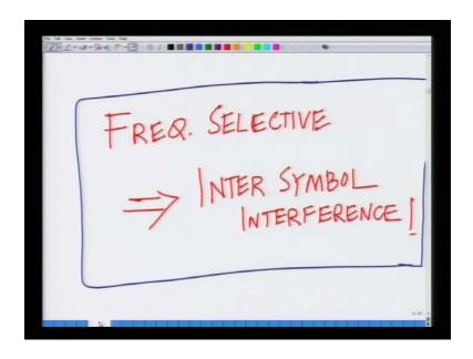
Specifically, we said if the channel is frequency selective that is, if the signal bandwidth is greater than the coherence bandwidth, then in time domain it means that the delay spread is greater than the symbol time, hence the channel results in inter symbol interference, which causes distortion at the receiver. So, frequency selectivity and the frequency domain corresponds to inter symbol interference in the time domain.
