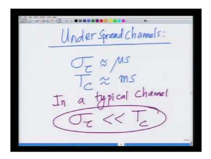
Let us now go to one final aspect in this channel characterization, which is that of under spread, this is under spread wireless channel, if you looked before, we said the delay spread of an outdoor wireless channel is approximately of the order of micro seconds. And the coherence time is approximately of the order of mille second, look at this, we looked at both the delay spread of the outdoor channel, and the coherence time.
