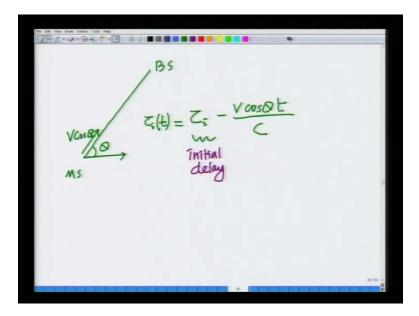
We said this Doppler or this velocity of the mobile results in a time varying delay, previously we had our delay fixed, which tau i. But now because the mobile is moving that delay itself is
