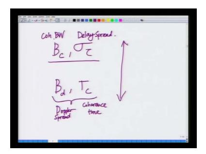
So, these two, so let we write them down here B c and coherence bandwidth, and the delay spread sigma tau are related to each other, this is coherence bandwidth, coherence bandwidth, and the delay spread are related to each other. And the Doppler spread, and coherence time these two are related to each other, Doppler spread and coherence time; I think it is essential to point out that sometime little confusing to think, that because the coherence word applies in both the bandwidth.
