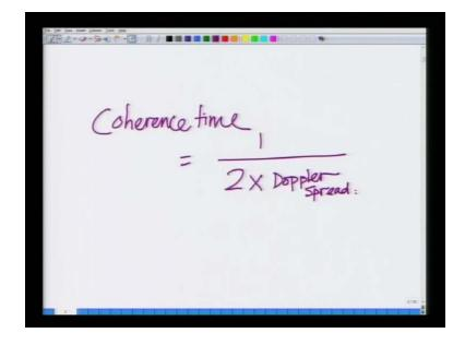
Let we write that clearly coherence time equals 1 over twice the Doppler spread of the channel, which is d d; let us do an example to understand this better.
