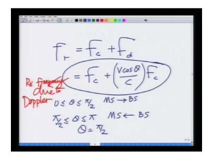
We also said, we also introduced the notion of Doppler resulting from a moving, moving mobile that is, has the mobile moves with the velocity V, the received carrier frequency changes. In particular that is given by this relation F c plus V cos theta over c times F c, where V cos theta over c F c is the Doppler shift, V is the velocity of mobile and theta is the angle of the velocity with line joining the base station and the mobile.
