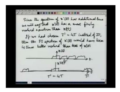
So, let us put this down since the spectrum of x dash t has additional lines, we will say that x dash t has a more finely resolved spectrum, then x of t and it became more finely resolved simply by changing the periodicity of the signal without changing the shape of the signal adding it with extra 0 space, and doubling the period from t from capital to capital t dash. If you wish you can go back to the definition and take a look this was the definition of t dash t with respect to t t.
