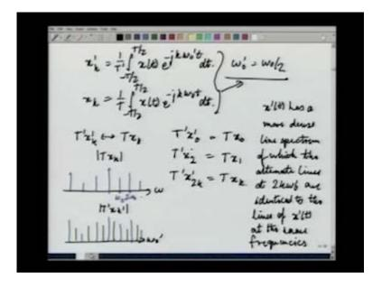
If you look at the equations we would finally get, it is the following we have x dash k equals integral one by T dash, sorry integral minus T by 2 to T by 2 x t not x dash t x t well x dash t also, but at anyway we can simplify to x t e to the minus j k omega naught
