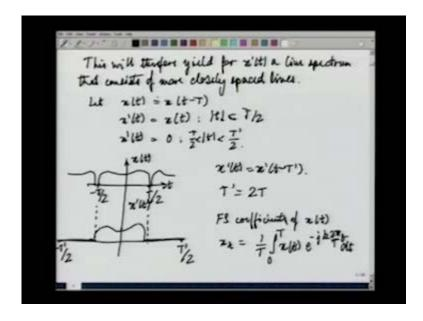
This will therefore yield for x dash t a line spectrum, that is or that consists of more closely spaced lines why simply, because for x dash of t not only is the fundamental frequency omega naught dash less than omega naught, which was the fundamental
