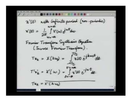
So, to summarize we have x dash t with infinite period that is to say non periodic alright, it has infinite period and is given by this is nothing but the synthesis equation or the inverse Fourier transform equation. What we have just discovered is the Fourier transform though we have actually landed up directly with the inverse Fourier transform.
