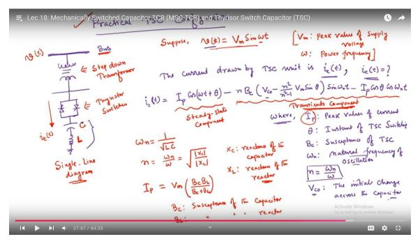
$$i_c(t) = I_P \cos(\omega t + \theta) - nB_C \left( V_{C_0} - \frac{n^2}{n^2 - 1} V_m \sin \theta \right) \sin(\omega_n t) - I_P \cos(\theta) \cos(\omega_n t)$$
