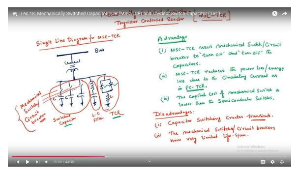
The capital cost of mechanical switch is lower than the semiconductor switches. So, therefore, between these two switchable capacitor options, one is TSC that is thyristor switched capacitor, another is mechanical switch capacitor that MSCTCR is advantageous as far as the cost or capital cost is concerned. So, these are the advantages.
