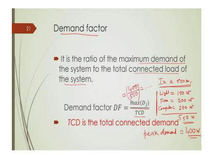
Now, we have certain indices to study; one is called demand factor. Demand factor is the ratio of maximum demand of the system to the total connected load ok. So, demand factor is the ratio of maximum demand to the total connected load. It means that if I give an example that let us say in a particular room, we have a number of appliances.
