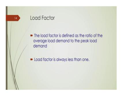
Now, I think I stopped at this point, where I discussed this load factor ok. So, load factor is one of the indices which is used for modeling electrical load ok and as I discussed in my last lecture, it is a ratio of the average load to the peak load demand or maximum load demand ok. So, load factor is always less than 1; why it is so, I discussed.
